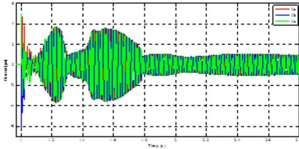
**Fig. 8** Waveform current in connection wind turbine to the main Grid without battery storage source.
