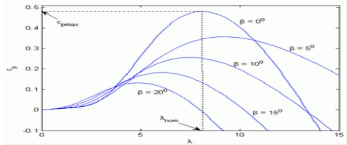
Fig. 2 Characteristic power efficiency in terms of edge speed and for various quantities of pitch angle [9]
