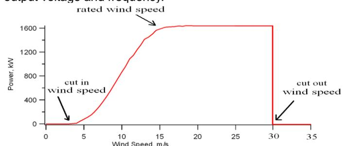
Fig. 3 Curve of allowable working range of wind turbine based on wind speed.
