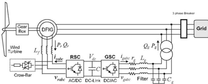
**Fig. 4** Schematic of simulated of connected wind turbine to the main Grid.
