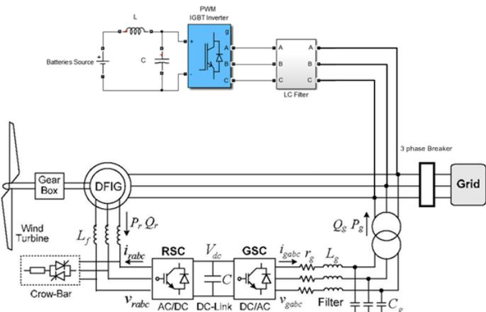
**Fig. 5** Schematic of simulated sample of connected wind turbine to the main Grid the presence of battery storage source.
