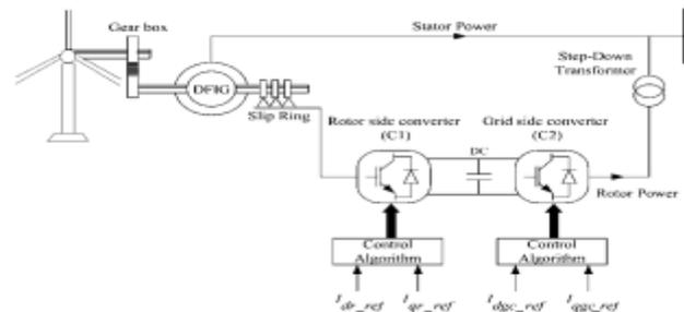
**Fig. 1** schematic of connected doubly fed induction generator to Main Grid
