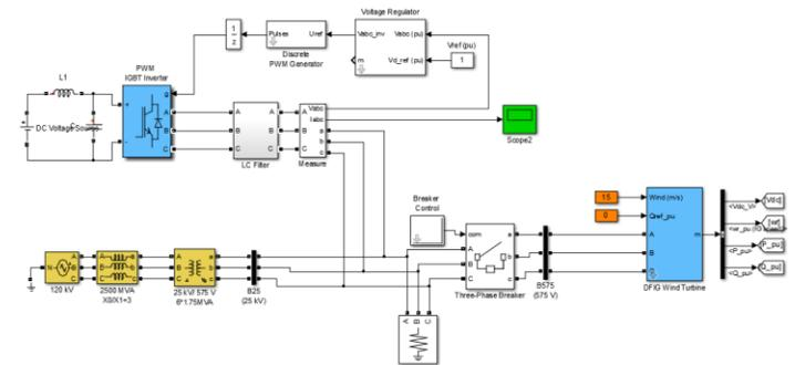
**Fig. 6** Simulation of connected wind turbine to the main Grid in MATLAB.
