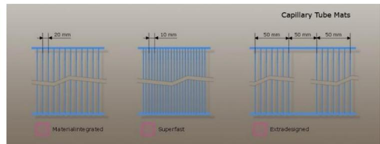
Fig. 1: capillary tube mats [3]
