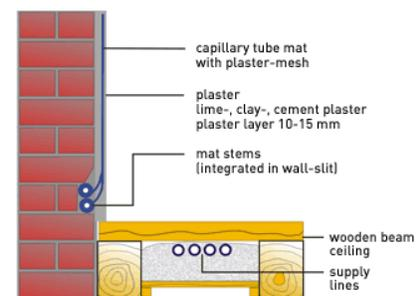
Fig. 2: capillary tube mats on walls [4]
