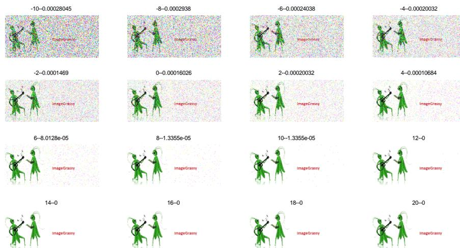
**Figure7.** Transmission of PNG Icon with varying Modulation Index
