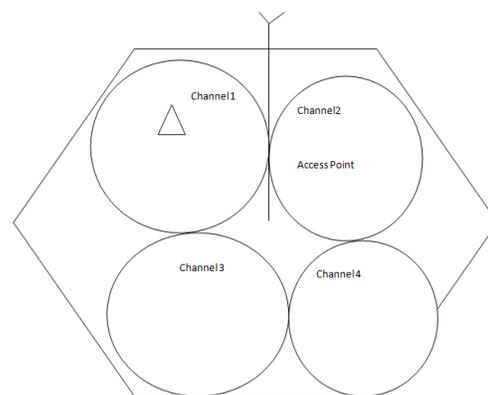
**Figure3.** Hexagonal cellular architecture
