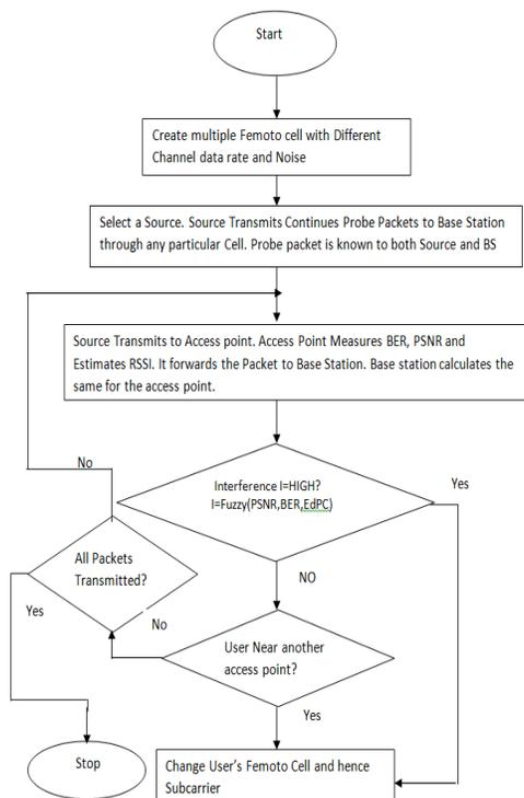
Figure4. Flow chart of fuzzy based resource allocation
