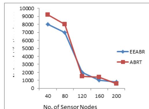
**Figure 5.** Number of sensor nodes Vs life time
