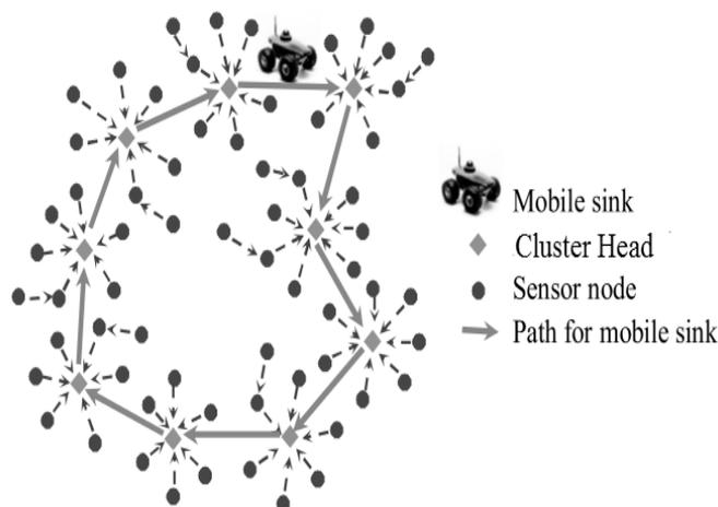
Figure 2. Sensor Network with mobile sink
