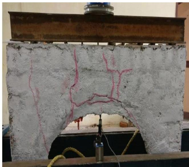
**Fig. 4. Failure behaviour of intrados strengthened arch.**
