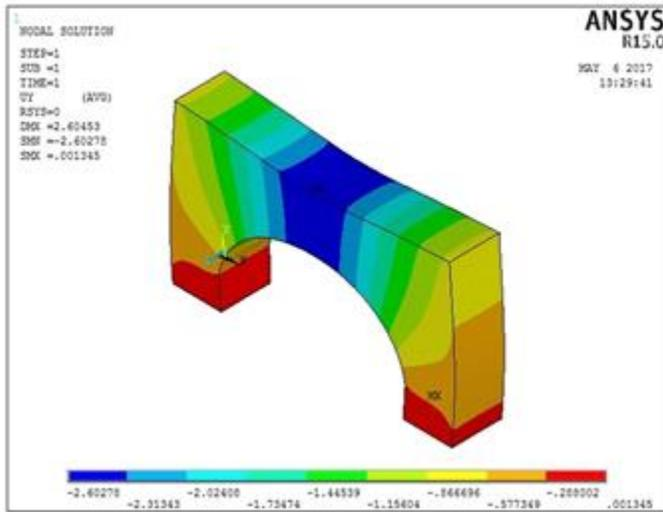
Fig. 8. Stress pattern of unstrengthened arch
