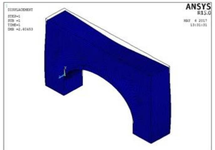
Fig. 11. Deformation shape of unstrengthened arch.
