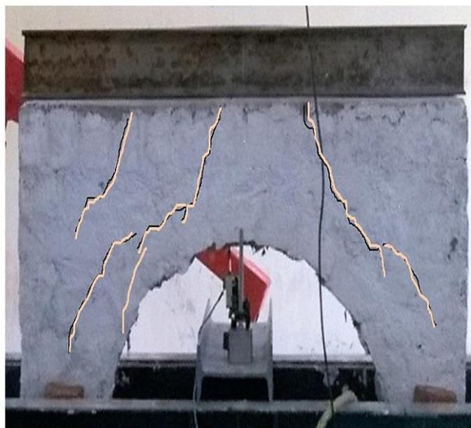
**Fig. 5. Failure behaviour of extrados strengthened arch**
