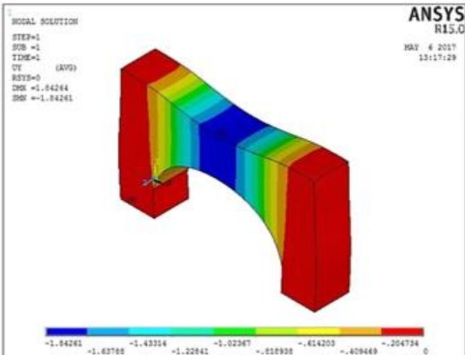
Fig. 9. Stress pattern of extrados strengthened arch.
