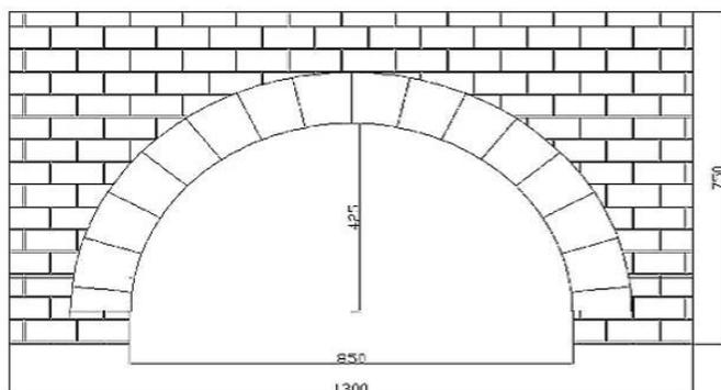
**Figure 1 Geometry of the masonry arch.**
