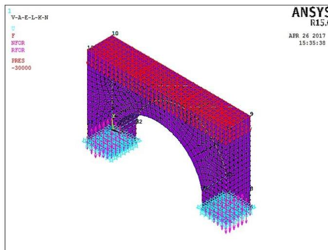
Fig. 7. Modelling of masonry arch using ANSYS
