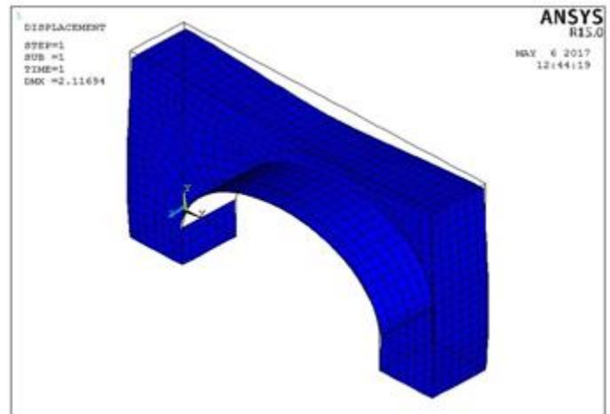
Fig. 12. Deformed shape of intrados strengthened arch.
