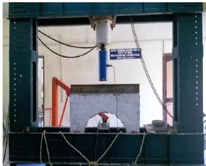
**Fig. 2. Test setup of masonry arch in loading frame.**
