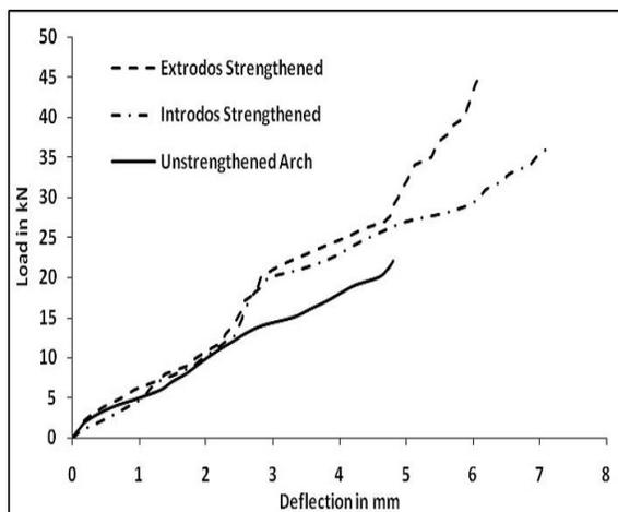
Fig. 6. Load - displacement of Unstrengthened and SRG strengthened arches
