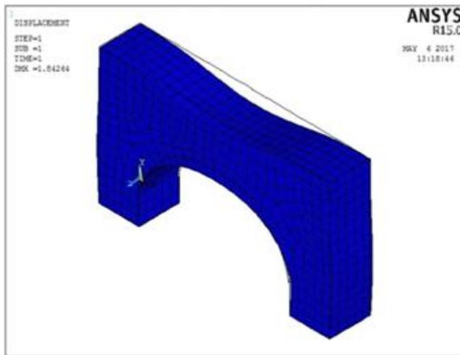
Fig. 13. Deformed shape of Extrados strengthened arch.
