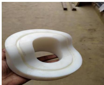
*Final Part of The Cam Plate After Milling Done by CNC L-MILL*
