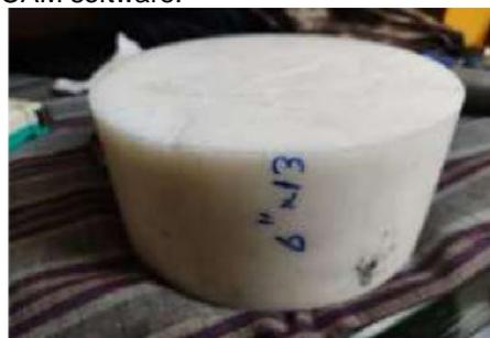
*Nylon Material to Make Cam Plate*
