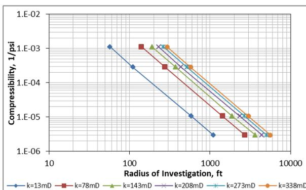
**Fig. 3.** The effect of compressibility and permeability on radius of investigation  $r_i$
