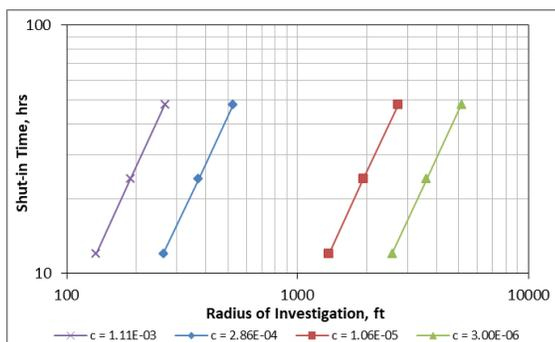
**Fig. 5.** The effect of compressibility and shut-in time on radius of investigation *r<sub>i</sub>*
