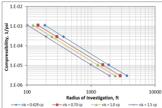
**Fig. 2.** The effect of compressibility and viscosity on radius of investigation  $r_i$
