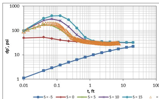
Fig. 1. The effect of skin factor on pressure derivative curve.
