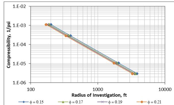
**Fig. 4.** The effect of compressibility and porosity on radius of investigation  $r_i$
