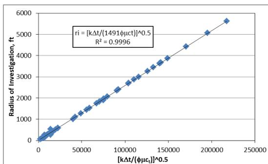
**Fig. 6.** Plot of *r<sub>i</sub>* vs.  $[k\Delta t/(\phi\mu ct)]^{0.5}$ .
