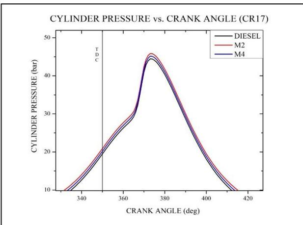
**Fig 4.** Combustion characteristics of various biodiesel blends and diesel
