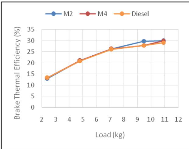
**Fig 3.** Variation of BTE with various engine loads
