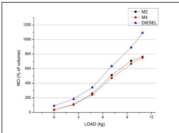
Fig 8. Variation of NO<sub>x</sub> with various engine loads
