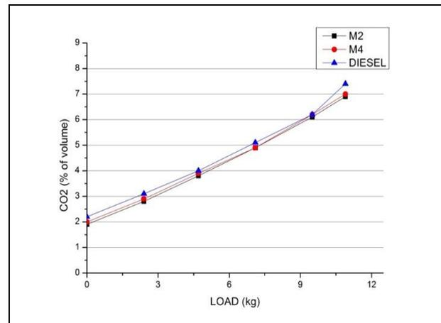
**Fig 6.** Variation of CO<sub>2</sub> with various engine loads
