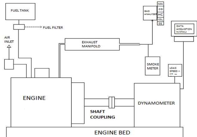
Fig 1. Engine setup layout
