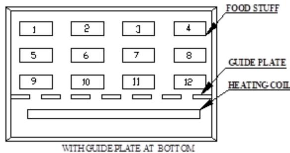
**Fig. 3** Experimental setup without booster heating coil guide plate and with the bottom guide plate
