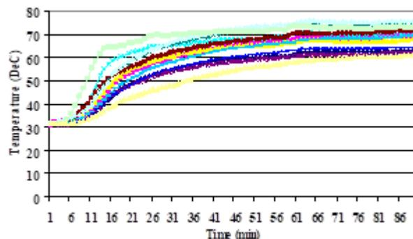
**Fig. 7** Temperature variation of foodstuffs (without guide plate)
