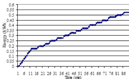
Fig. 12 Cumulative energy consumption of display cabinet (Middle guide plate)
