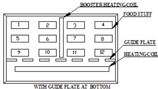
Fig. 14 Display cabinet with guide plate at the bottom
