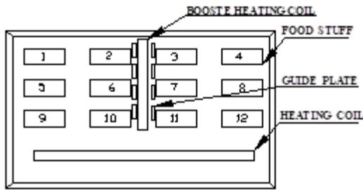
Fig. 10 Guide plate at middle
