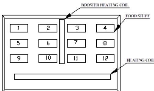
**Fig. 6** Experimental setups without guide plate
