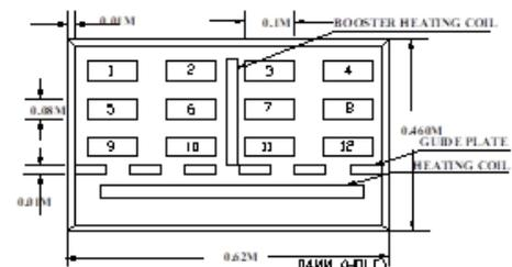
Fig 1.0 Geometry of the display cabinet
