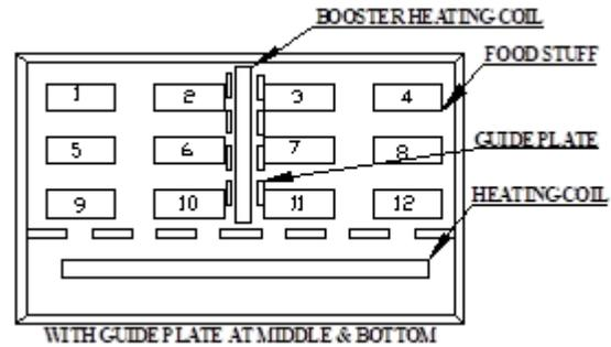
**Fig 18** Display cabinet with guide plate at middle
