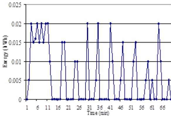
**Fig 21** Energy consumption of display cabinet (Bottom Guide plate)
