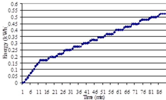
**Fig .16** Cumulative energy consumption of display cabinet (Bottom Guide plate)
