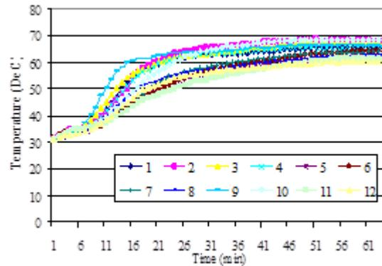
**Fig 19** Temperature variation of foodstuff (Middle and Bottom guide plate)
