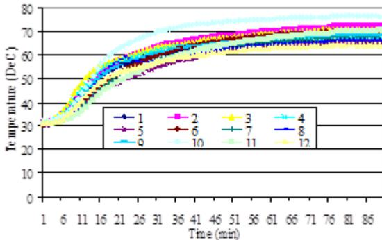
Fig. 11 Temperature variation of food stuff (guide plate at middle)
