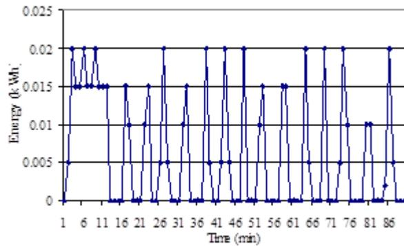
Fig. 13 Energy consumption of display cabinet (Middle guide plate)
