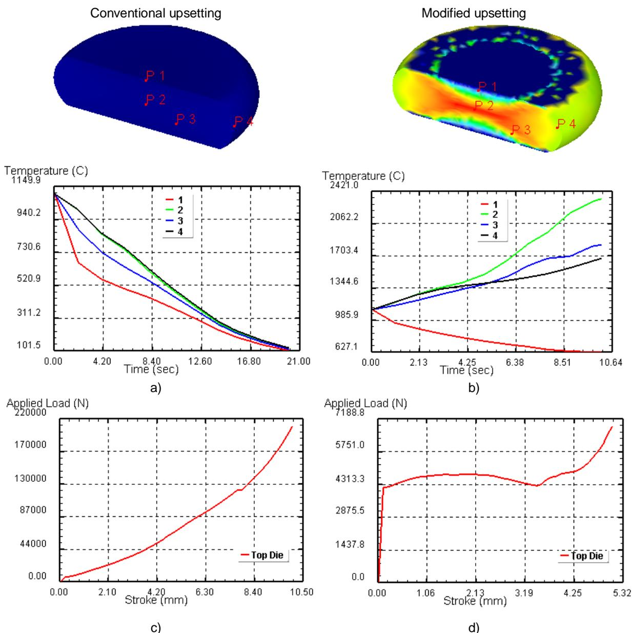
**Figure 2.** Load-stroke and temperature variation during the upsetting process.
