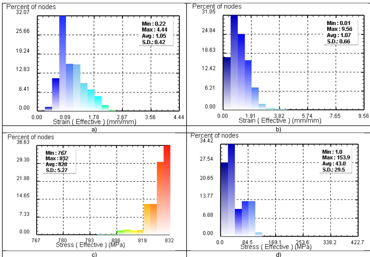
**Figure 4.** Effect of die movement on the (a-b) effective strain distribution and (c-d) effective stress distribution.
