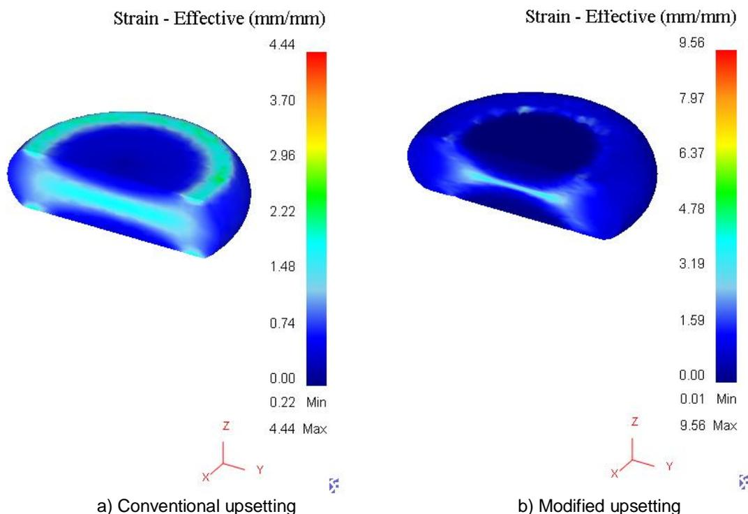
**Figure 1.** Deformed short cylinder at 1100 °C and die speed of 0.5mm/sec.
