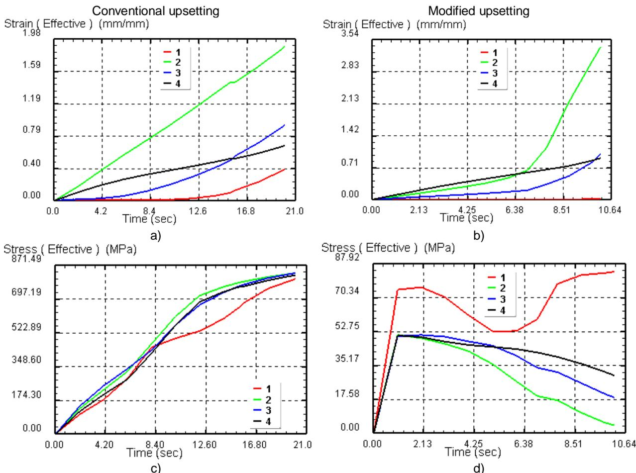
Figure 3. Effect of die movement on (a-b) the effective strain distribution and (c-d) effective stress distribution.
