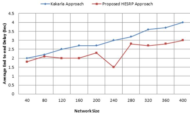
**Fig.5. Comparison of End to end delay with Network size**
