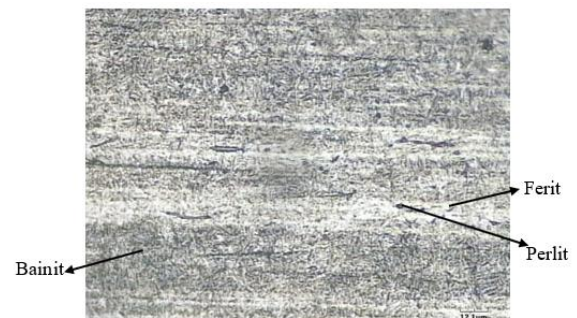
Figure 11. ASSAB 705 M Steel After Austempering Process at 350 ° C
