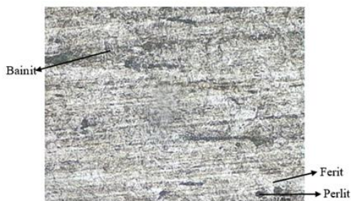
Figure 10. ASSAB 705 M Steel After Austempering Process at
