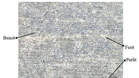
Figure 11. ASSAB 705 M Steel After Austempering Process at 350 ° C
