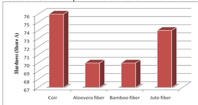
**Fig. 2.** Comparison of average hardness of different fiber sheets
