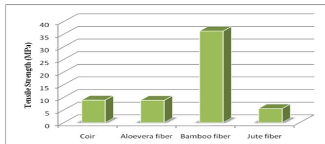
**Fig. 1.** Comparison of average Tensile strength of different fiber sheets
