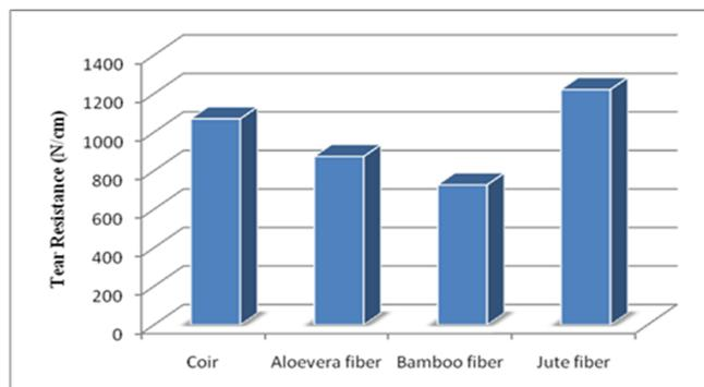
**Fig. 3.** Comparison of average tear resistance of different fiber sheets
