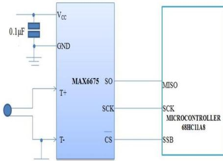
**Fig. 6** Interfacing of Thermocouple
