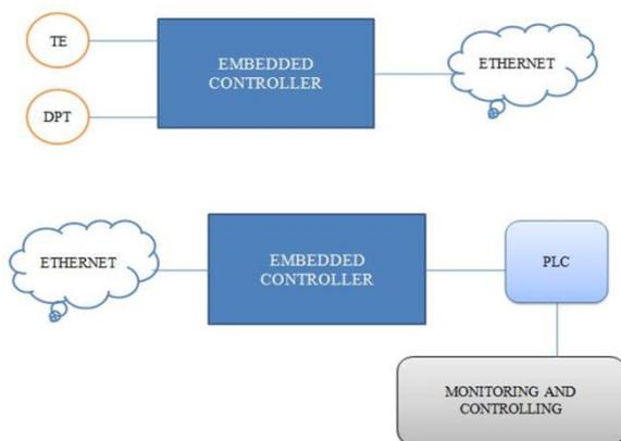
Fig. 1 Block Diagram of Sensor Monitoring
