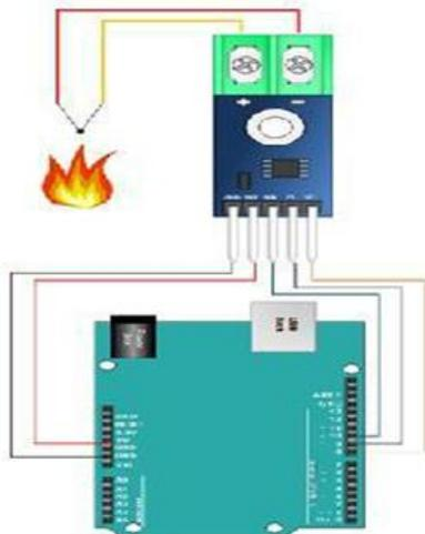
**Fig. 2** Interfacing Thermocouple with Arduino
