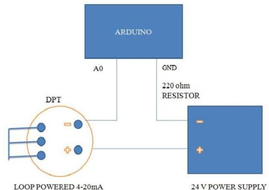
**Fig. 5** Interfacing of DPT
