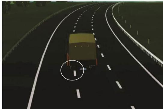
**Fig. 13.** The partial lane departure of SUT at NSE Rawang.
