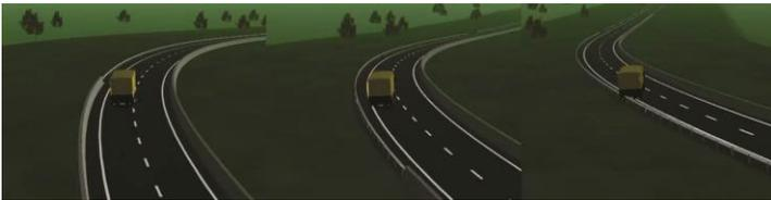
**Fig. 7.** Over-steering behavior of the tested SUT at NSE N5 Menora Tunnel – Sungai Perak.
