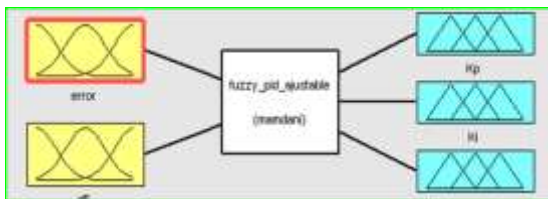
Fig.5(c). The developed in MATLAB simulink hybrid fuzzy algorithm with two input and three outputs
