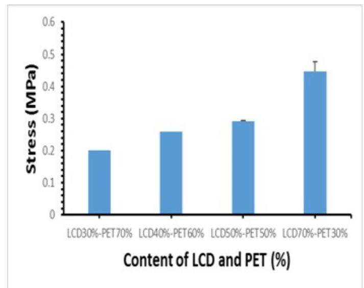
**Figure 10.** Average variation of tensile strength of specimens in each formulation.
