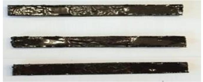
Figure 6. Specimens prepared from LCD-PET composite plate for bending test.
