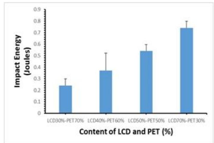
**Figure 13.** Comparison of Impact energy of LCD-PET composite formulations and also average variation of specimens in each formulation of LCD-PET composite material.
