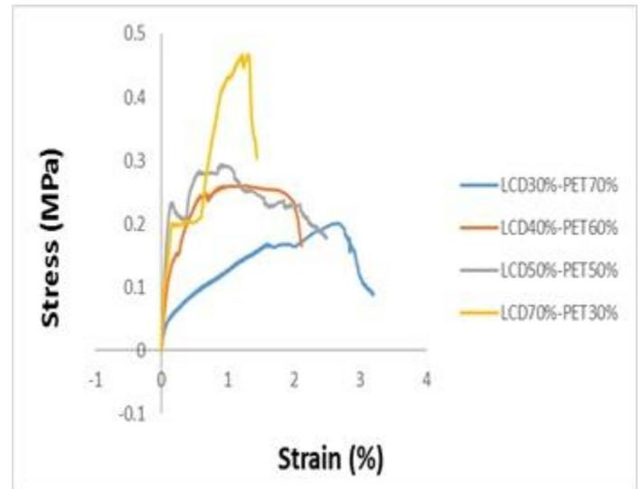
**Figure 9.** Comparison of stress-strain graph for tensile strength of LCD30%-PET70%, LCD40%-PET60%, LCD50%-PET50% and LCD70%-PET30% composite material.
