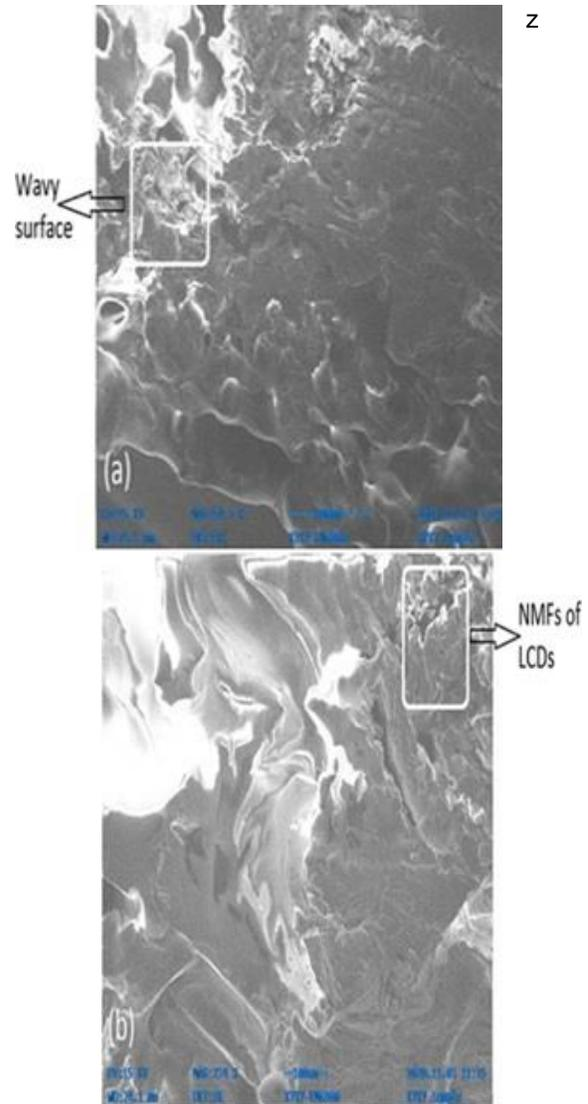
**Figure 15.** SEM image of fracture surface of LCD50%-PET50% (a) fracture surface MAG: 54.7 X (b) fracture surface MAG: 274 X.
