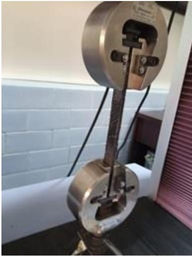
Figure 3. Specimen gripped in UTM.
