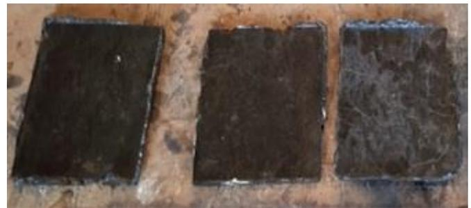
**Figure 1.** LCD-PET composite plate formed from NMFs of LCDs and PET contents.
