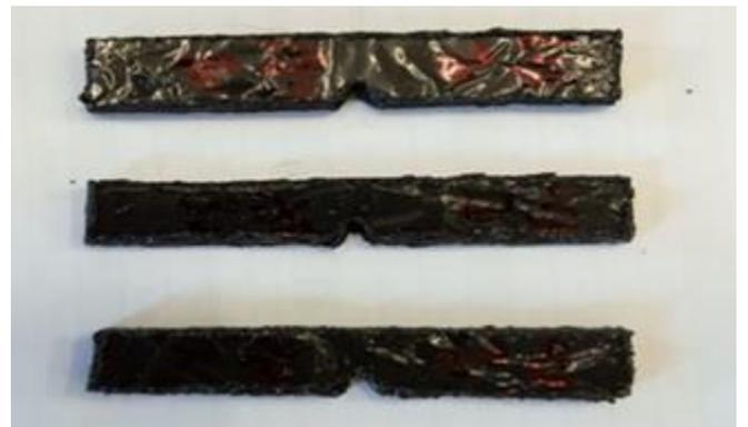
Figure 8. Specimens cut from LCD-PET composite plate for impact testing.
