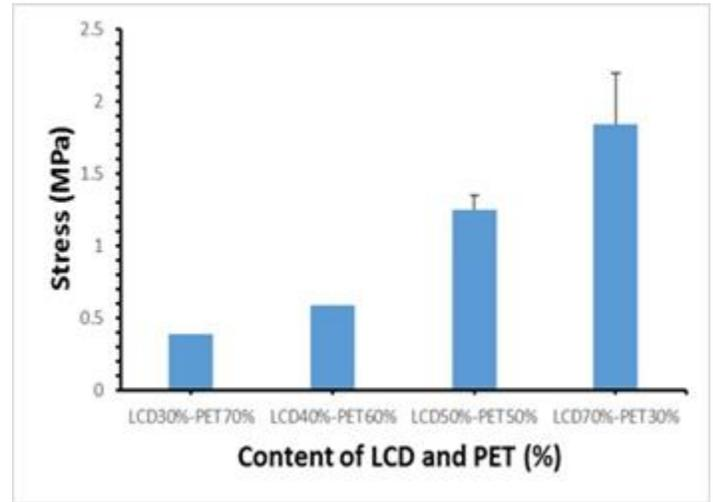
**Figure 12.** Average variation of bending strength of specimens in each formulation.
