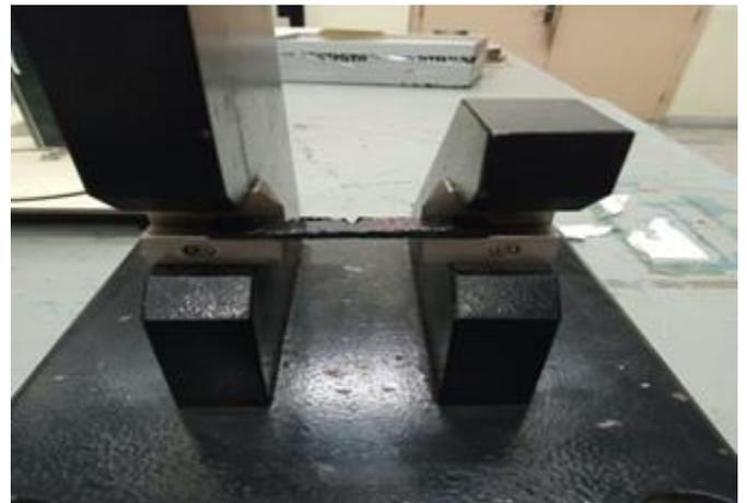
Figure 7. Specimen on anvil of charpy apparatus for impact testing.
