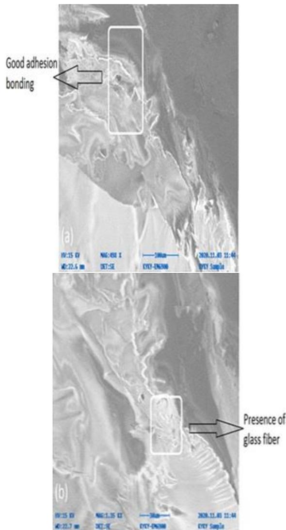
**Figure 14.** SEM image of fracture surface of LCD70%-PET30% (a) fracture surface MAG: 498 X (b) fracture surface MAG: 1.35 KX.
