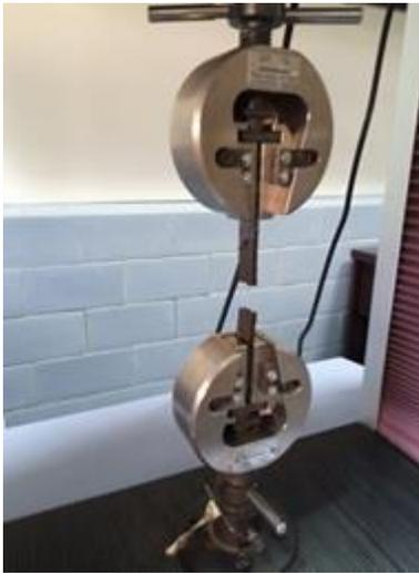
Figure 4. Specimen break under load during tensile testing.
