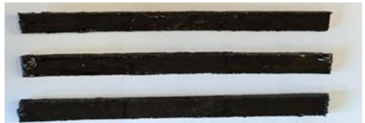
**Figure 2.** Specimens prepared from LCD-PET composite plate for tensile testing.
