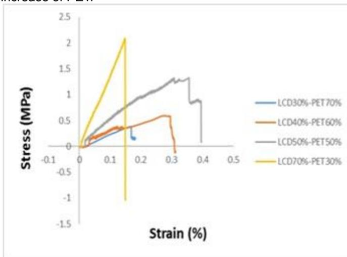
**Figure 11.** Comparison of stress-strain graph for bending strength of LCD30%-PET70%, LCD40%-PET60%, LCD50%-PET50% and LCD70%-PET30% composite material.
