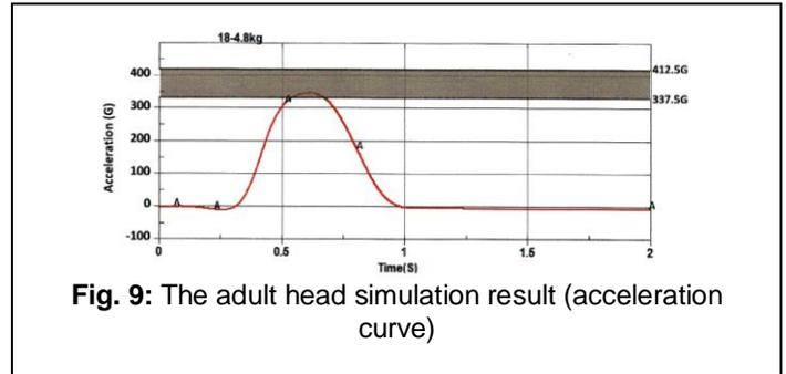
Fig. 9: The adult head simulation result (acceleration curve)
