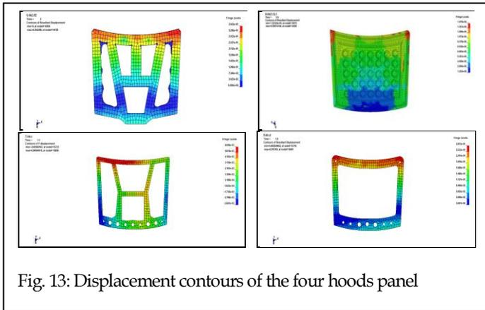
Fig. 13: Displacement contours of the four hoods panel
