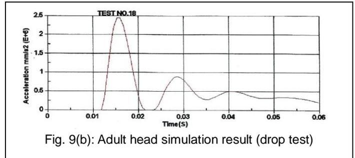
Fig. 9(b): Adult head simulation result (drop test)
