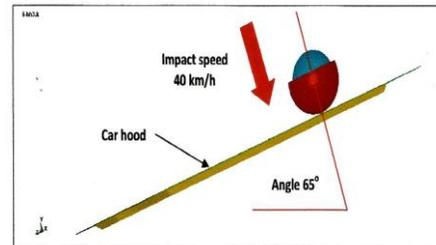
Fig 5: Head-hood impact test condition
