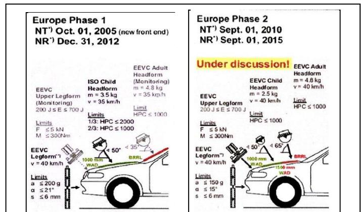
Fig.4: Car hood-head impact test (EU Phase 1, 2). [11]
