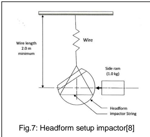
Fig.7: Headform setup impactor[8]
