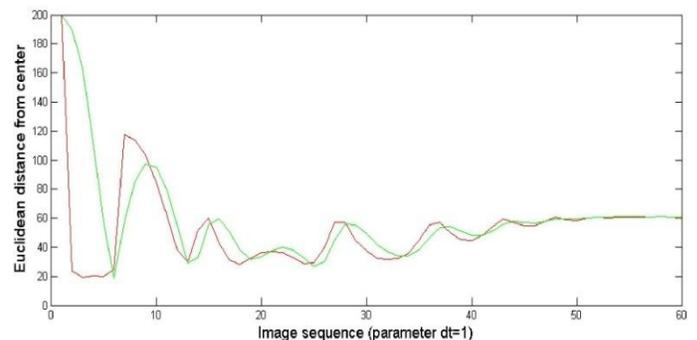
Same as previous representation, the red line represents the extracted object centre, while green line represents the Kalman Filter estimated object centre. Figure (6.4): Response of algorithm with shift of object coordinates (dt =100)
