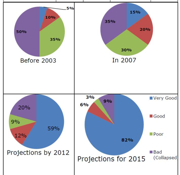
**Fig. 1 Current and Projected Conditions (Due to Intervention) of the Nigeria Road Network [3]**
