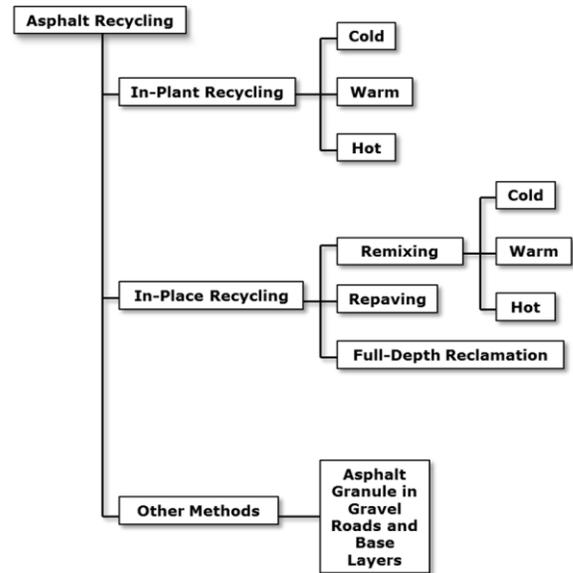
Fig. 4 Methods of Asphalt Recycling [34]
