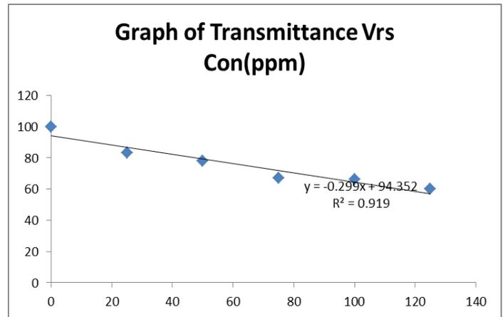
**Fig.2.** Graph of Transmittance vrs Concentration (ppm).
