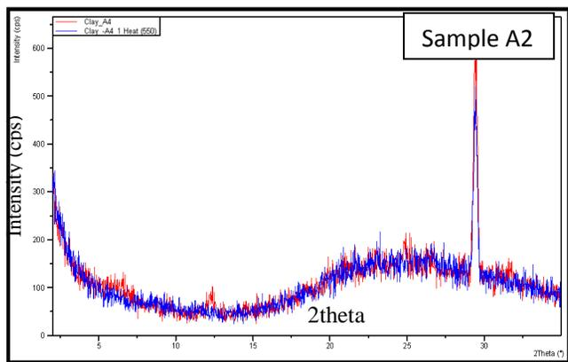
Fig.4: XRD patterns of clay fractions (<0.002 mm) of sample A2.
