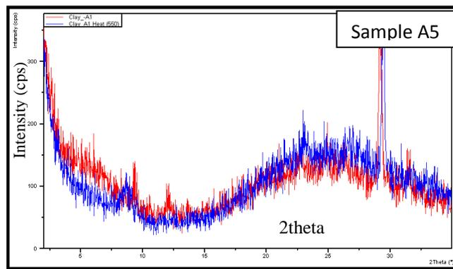
Fig.6: XRD patterns of clay fractions (<0.002 mm) of sample A5.
