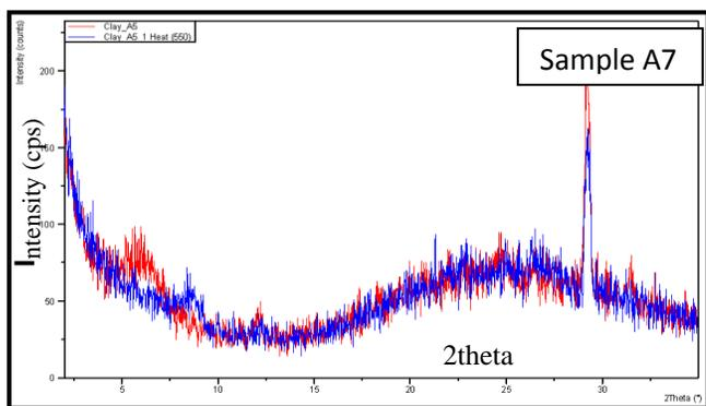
**Fig. 8:** XRD patterns of clay fractions (<0.002 mm) of sample A7.
