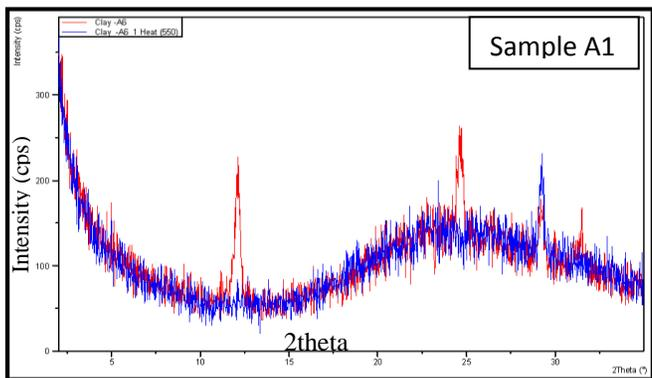
Fig.5: XRD patterns of clay fractions (<0.002 mm) of sample A1.
