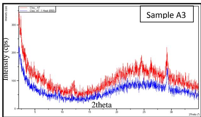
Fig. 3: XRD patterns of clay fractions (<0.002 mm) of sample A3.
