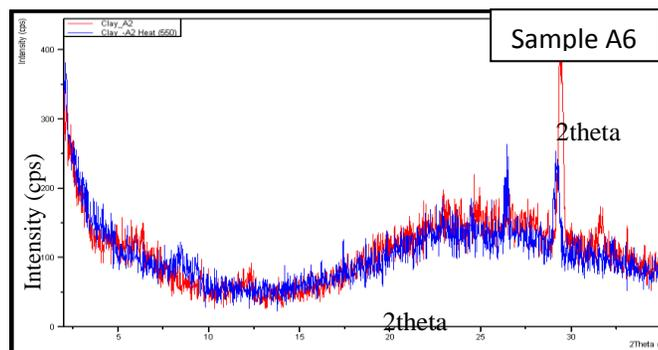
Fig. 7: XRD patterns of clay fractions (<0.002 mm) of sample A6.
