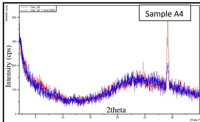
Fig. 2: XRD patterns of clay fractions (<0.002 mm) of sample A4.
