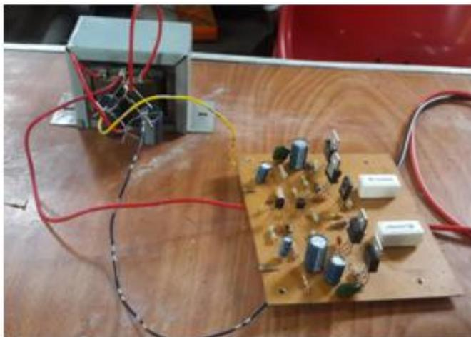
**Fig1.12** Test of output power amplifier and power supply
