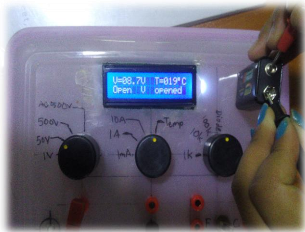
Fig.11 Test and result of voltage sensing
