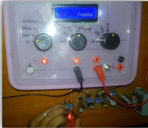
Fig.17 Test and result of frequency sensing
