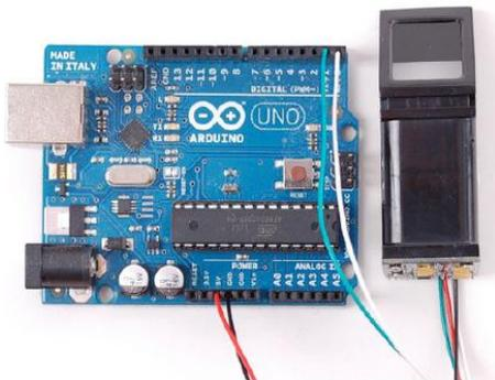
**Fig- Adafruit optical fingerprint sensor**
