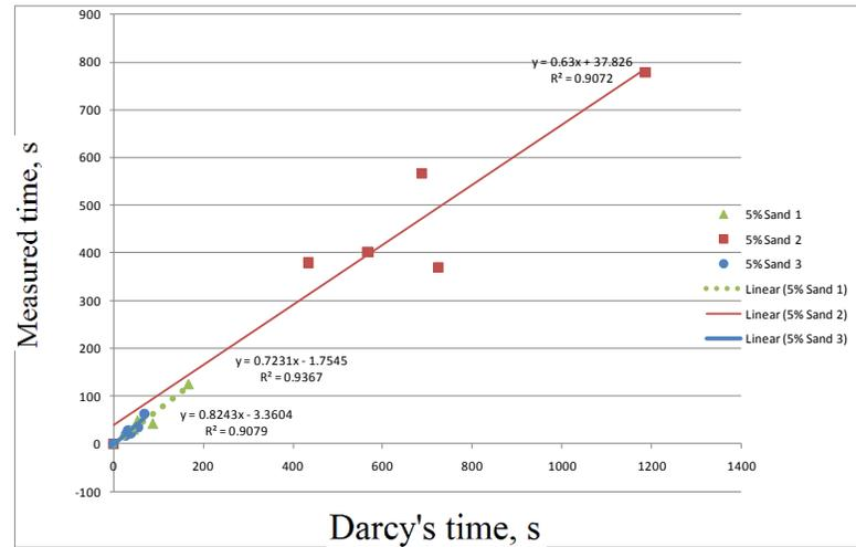
**Figure 5.** Comparison of measured time with Darcy's time for 5% brine solution
