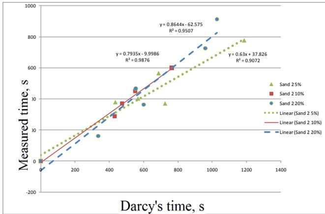
**Figure 3.** Comparison of measured time with Darcy's time for sand 2
