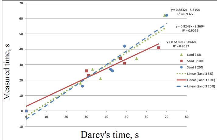
**Figure 4.** Comparison of measured time with Darcy's time for sand 3
