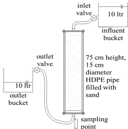
Figure 1. Schematic diagram of Lab-Model
