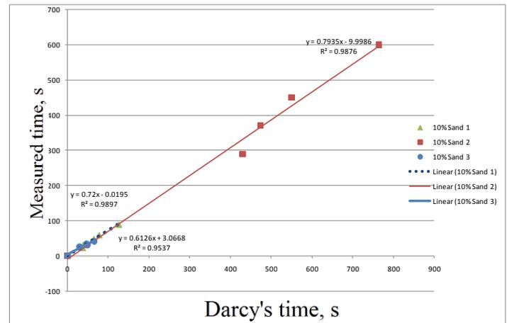
**Figure 6.** Comparison of measured time with Darcy's time for 10% brine solution
