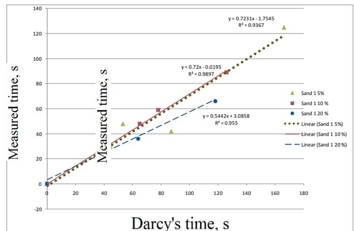
Figure 2. Comparison of measured time with Darcy's time for sand 1
