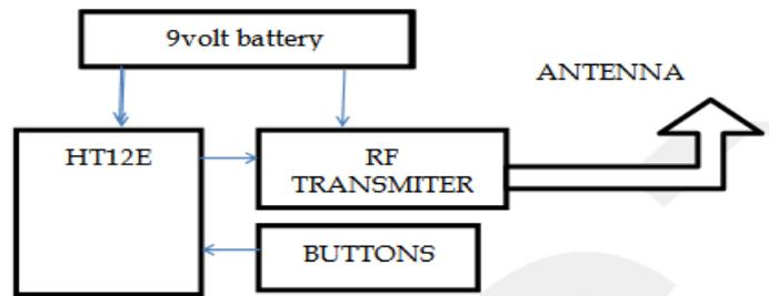
Figure 3: Block Diagram Radio Frequency Transmitters
