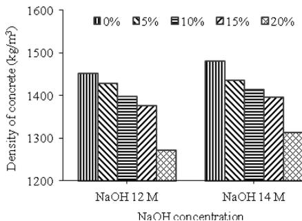
Fig. 12. Effect of NaOH concentration on density
