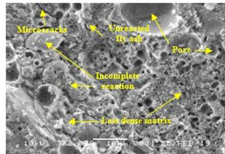
**Fig. 19.** Microstructure test results on mixed LGC at 10% kaolin and 12M NaOH
