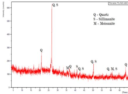
Fig. 3. X-ray diffraction pattern of fly ash
