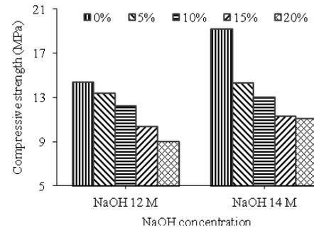
Fig. 14. Effect of NaOH concentration on compressive strength
