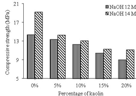
Fig. 13. Effect of kaolin percentage on compressive strength
