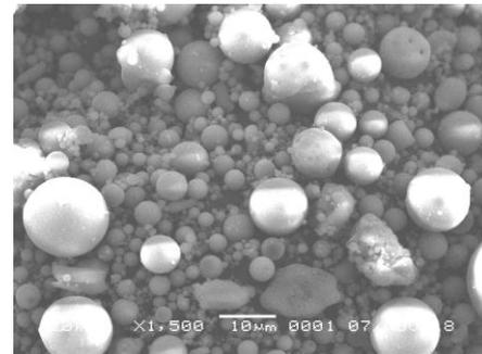
**Fig. 1. The microstructure of fly ash**
