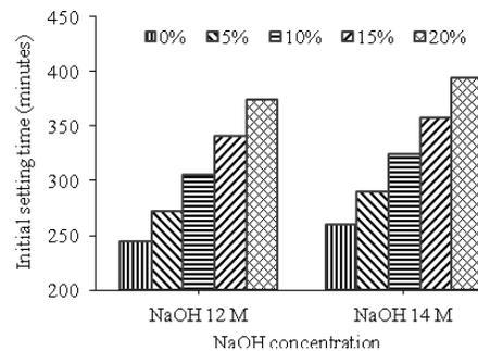
Fig. 9. Effect of NaOH concentration on initial setting time
