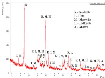
Fig. 4. X-ray diffraction pattern of kaolin
