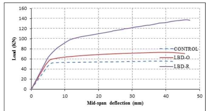
**Fig. (11)** Load –Deflection Curves For Tested Beams
