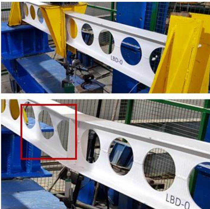
**Fig.(9).** Failure Mode In LBD-O
