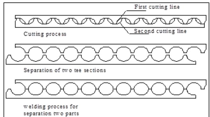
Fig.(1). Fabrication procedure Of Cellular Beams
