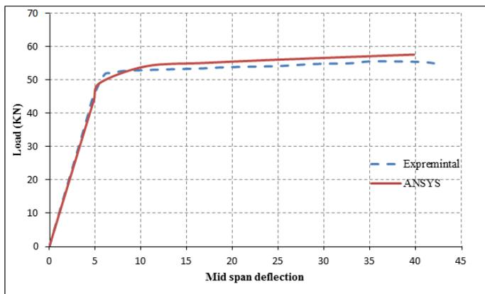
**Fig. (17). Load-Deflection Curves Of Control Beam**
