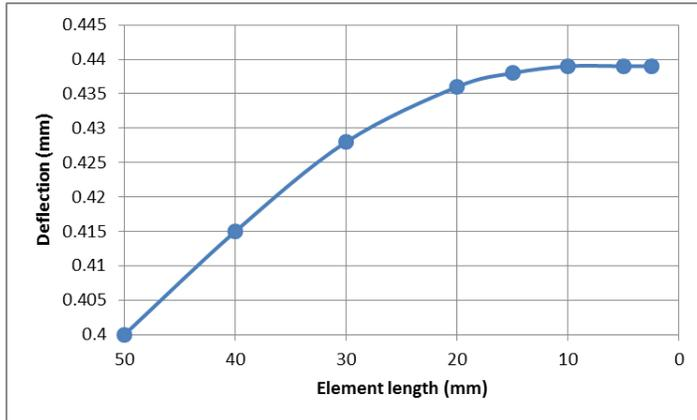
**Fig.(16). Testing Element Length**
