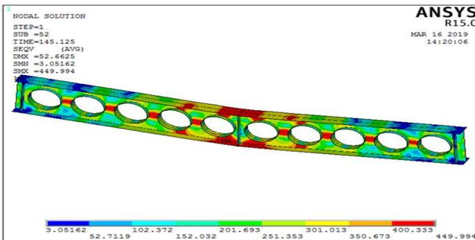
Fig.(22). Deformation Shape Of LBD-R
