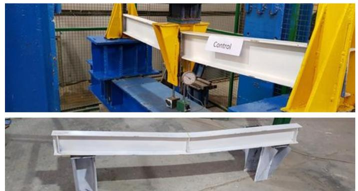
**Fig.(7). Failure Mode In Control Beam**
