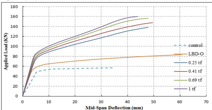
Fig.(22). Load-Deflection Response for Different Strengthening Thickness
