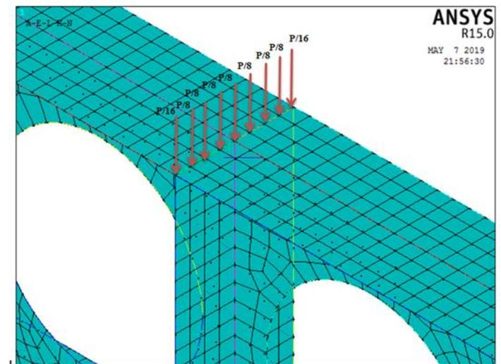
**Fig. (15). Applied Load By ANSYS**
