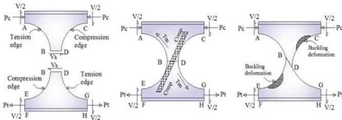
**Fig.(8).** Web-Post Buckling Mechanism
