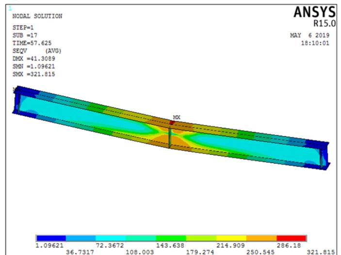
**Fig.(20). Deformation Shape Of Control Beam**
