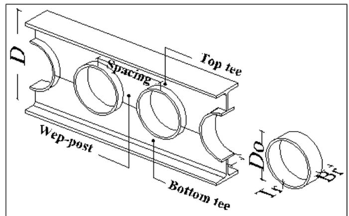
Fig.(2). Steel Ring Stiffeners Around Web-Opening
