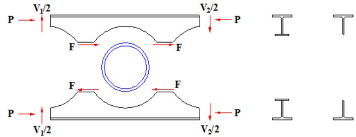
**Fig. (13) Effect Of Steel Ring On Cellular Beams Behaviour**
