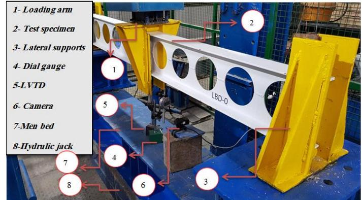
**Fig.(6). Test Procedure**
