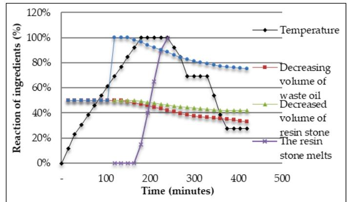
Figure 5. Graph of behavior change in asphalt material
