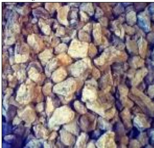
Figure 2. Coal mine waste (resin stone)
