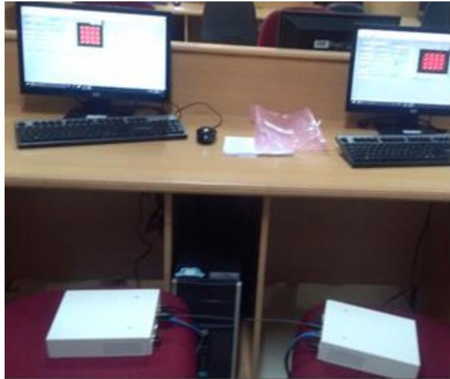
**Fig. 4.** Transmitter (Right side) and Receiver (Left side) connected to two NI 2920 USRP devices
