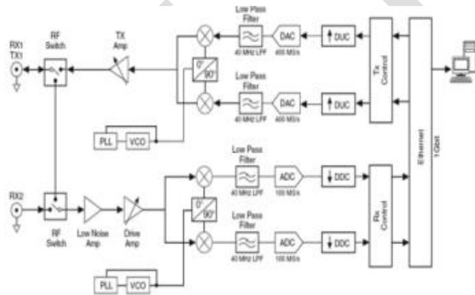
Fig 2. NI USRP 2920 System Block diagram
