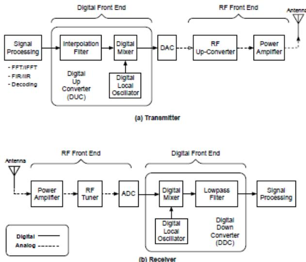
Fig. 1. System block diagram - NI 2920 (Image Courtesy [3])
