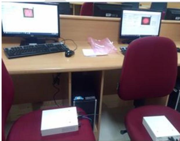
**Fig. 5.** Transmitter and receiver in NLOS condition.
