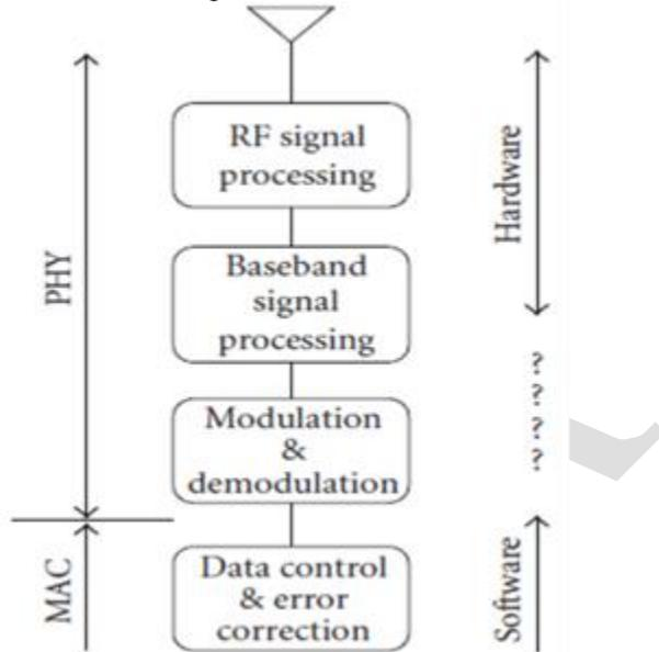
Fig 3. Hardware and Software Processing in SDR
