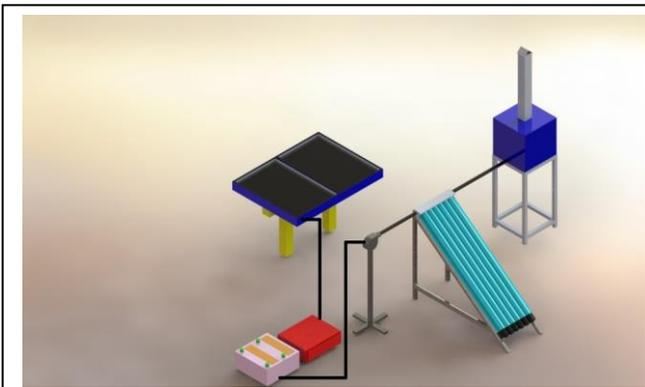
Fig. 1. Schematic diagram of Photovoltaic Thermal hybrid Solar Dryer assisted with ETC.
