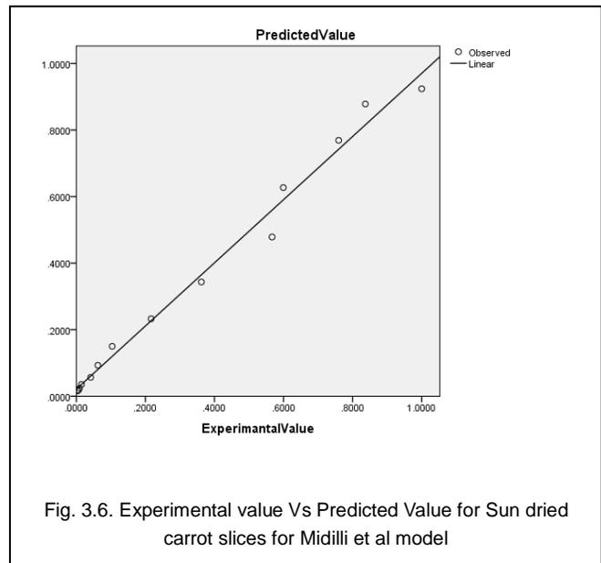
Fig. 3.6. Experimental value Vs Predicted Value for Sun dried carrot slices for Midilli et al model
