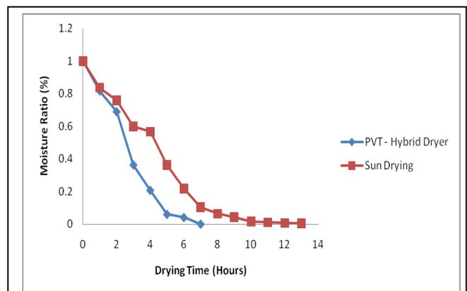
**Fig. 3.2. Moisture Ratio Vs Drying Time for PVT – Hybrid Solar Dryer and Sun Drying**
