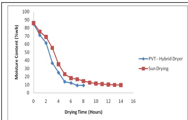
**Fig. 3.1. Moisture Content Vs Drying Time for PVT – Hybrid Solar Dryer and Sun Drying**
