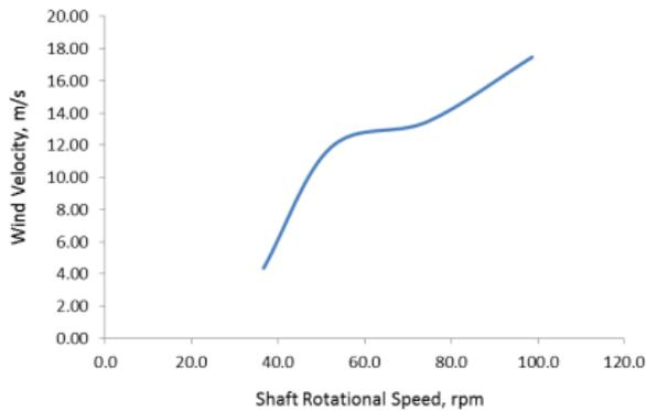
Fig. 6. Shaft rotational speed with respect to wind velocity.
