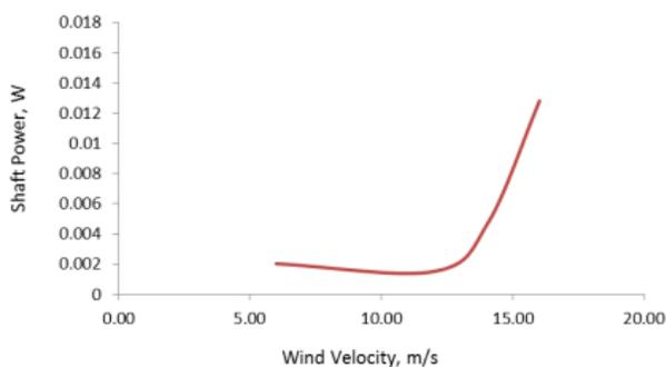
Fig.7. Shaft power output with respect to the wind velocity
