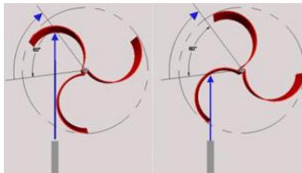
Fig.1. Layout of the Savonius blades
