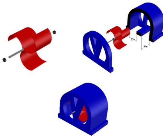
Fig. 3. Turbine blade housing assembly
