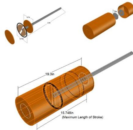
Fig. 4. Air pump components and assembly
