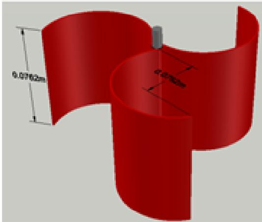
Fig.2. Turbine blade profile
