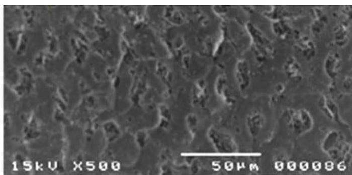
**Fig. 1.** SEM micrograph of acid activated *Canarium ovatum* Engl. Shells activated carbon
