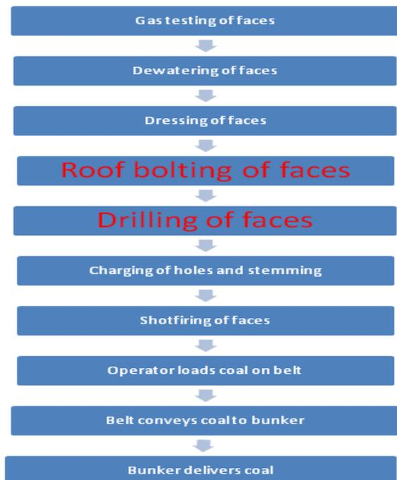
In mining process after dressing operation of the face, roof bolting is being done to support the roof. Drilling of face is being done to charge the holes by explosive and blasted to produce coal.
