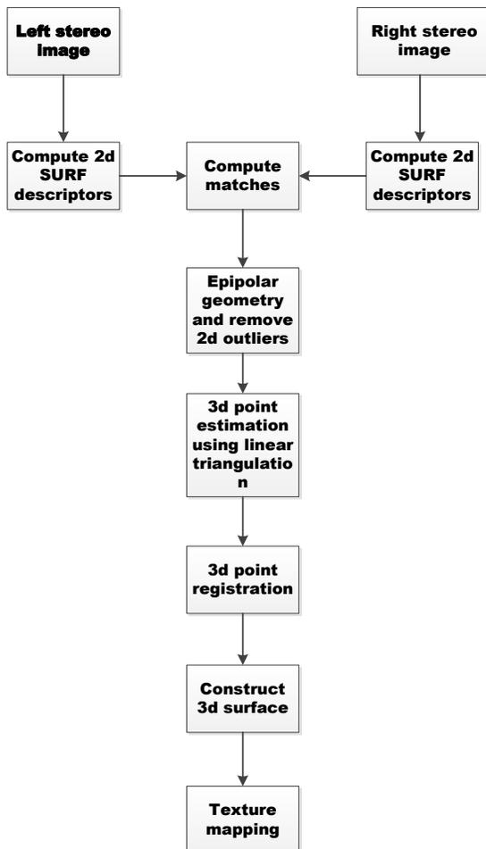
Figure.1 3d Reconstruction system using SURF
