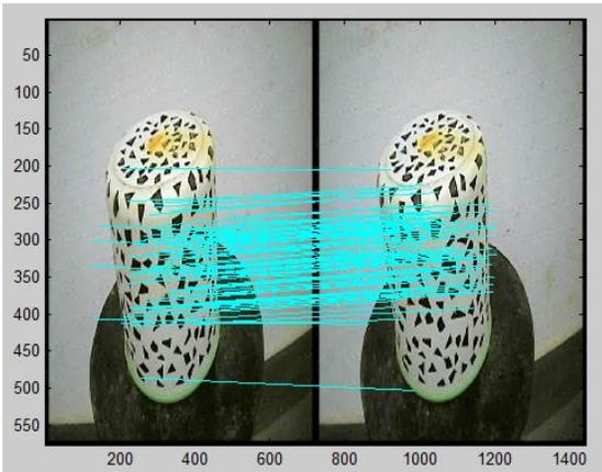
Figure.3 Surf descriptor matches with outliers removed
