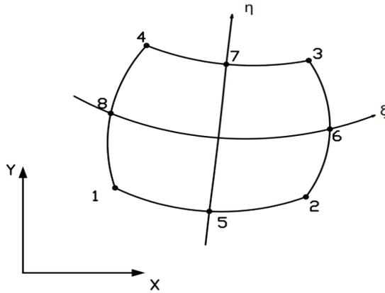
Fig.3: PLANE183 Geometry
