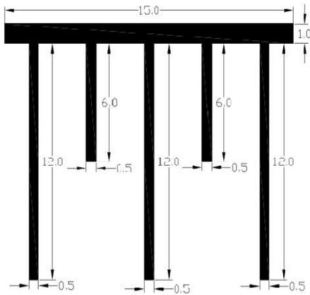
(g) Z3 – Alternate 12 m and 6 m pile length
