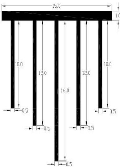
(h) V1 – Exterior – 10 m, interior – 12 m and middle pile length – 16 m
