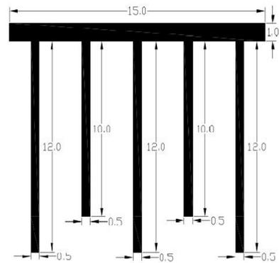
(f) Z2 – Alternate 12 m and 10 m pile length
