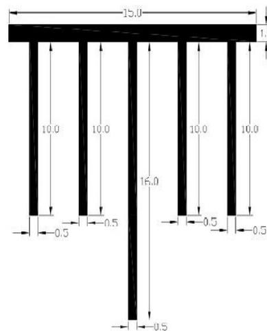
(l) T1 – Middle pile length – 16 m and other pile length - 10 m
