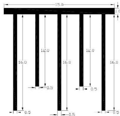
(e) Z1 – Alternate 16 m and 12 m pile length
