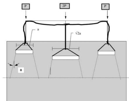
**Fig.1:** Redistribution of loads in a frame due to soil–structure interaction.
