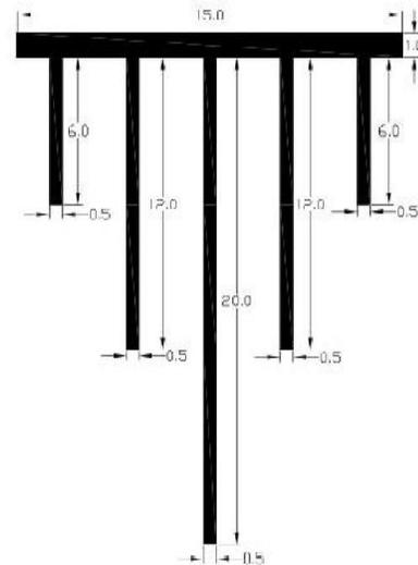
(k) V4 -- Exterior – 6 m, interior – 12 m and middle pile length – 20 m
