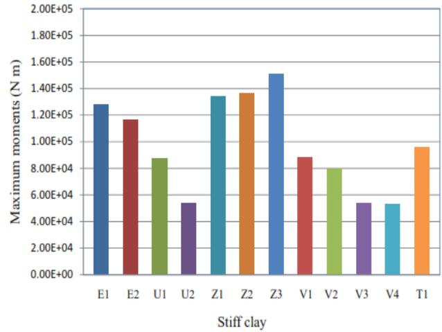
**Fig.8:** Maximum moments on frame along with stiff clay
