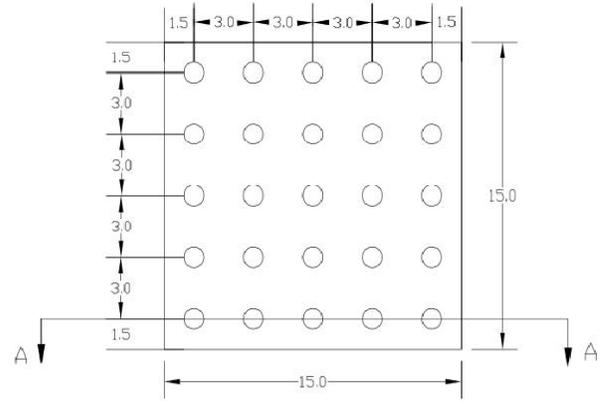
Fig.4: Plan of the building along with piles (All dimension are in m)
