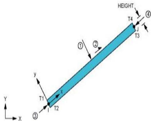
Fig.2: BEAM3 (2-D Elastic Beam) Geometry
