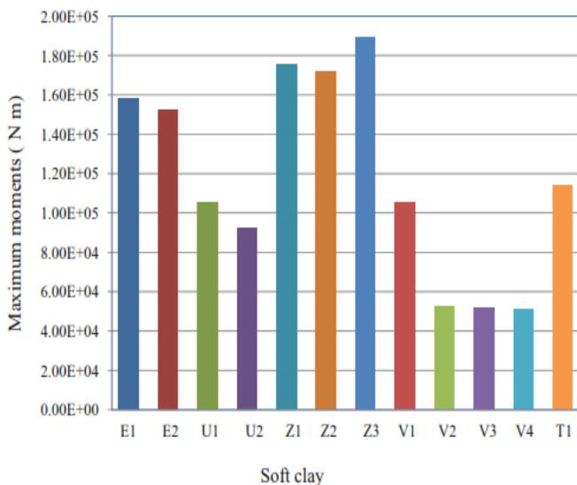
**Fig.7:** Maximum moments on frame along with soft clay
