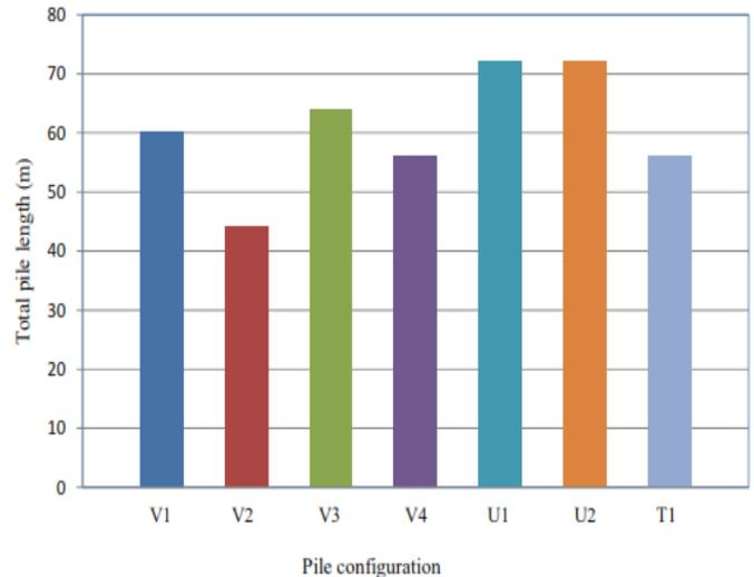
Fig.13: Total pile length for V-shape, U-shape and T-shape pile configurations
