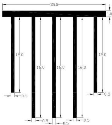
(c) U1 – Exterior and interior pile length 12 m and 16 m respectively
