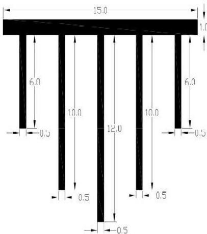
(i) V2 – Exterior – 6 m, interior – 10 m and middle pile length – 12 m
