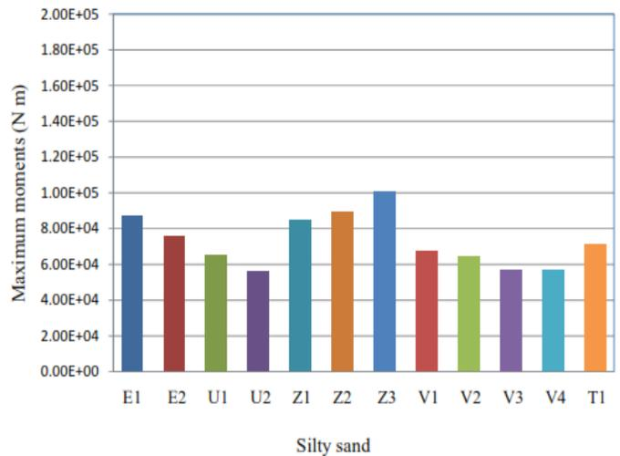
**Fig.9:** Maximum moments on frame along with silty sand
