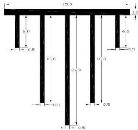
(j) V3 -- Exterior – 6 m, interior – 16 m and middle pile length – 20 m
