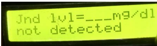
Fig 13: Jaundice level and duration display's in Receiver Section
