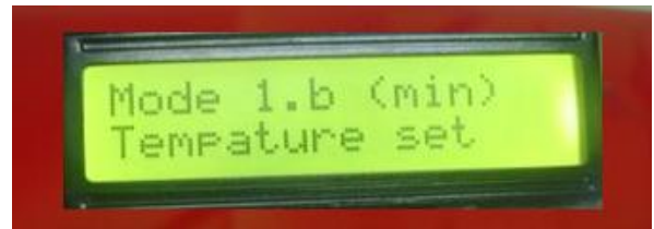
Fig 21: Minimum temperature setting mode display of the room at the Transmitter Section
