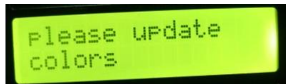
Fig 8: Receiver side LCD display "Please Update colors" The LCD displays "Please Update colors" as shown in Figure 8 when the key is pressed.
