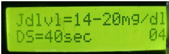
Fig 11: Jaundice level and duration display for color 2 at the Receiver Section
