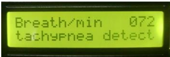
Fig 24: Display of respiration count per minute and detected tachypnea at the Receiver Section
