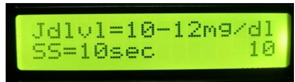
Fig 9: Jaundice level and duration display for color 0 at the Receiver Section
