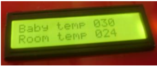
Fig 16: Temperature display of room and baby at the Receiver Section
