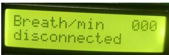
Fig 27: LCD display when the peizo sensor is disconnected from the baby.
