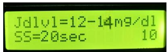
Fig 10: Jaundice level and duration display for color 1 at the Receiver Section
