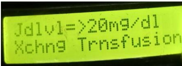
Fig 12: Jaundice level and duration display for color 3 at the Receiver Section
