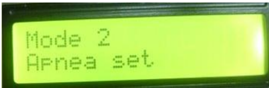
Fig 25: Apnea setting mode display at the Transmitter Section
