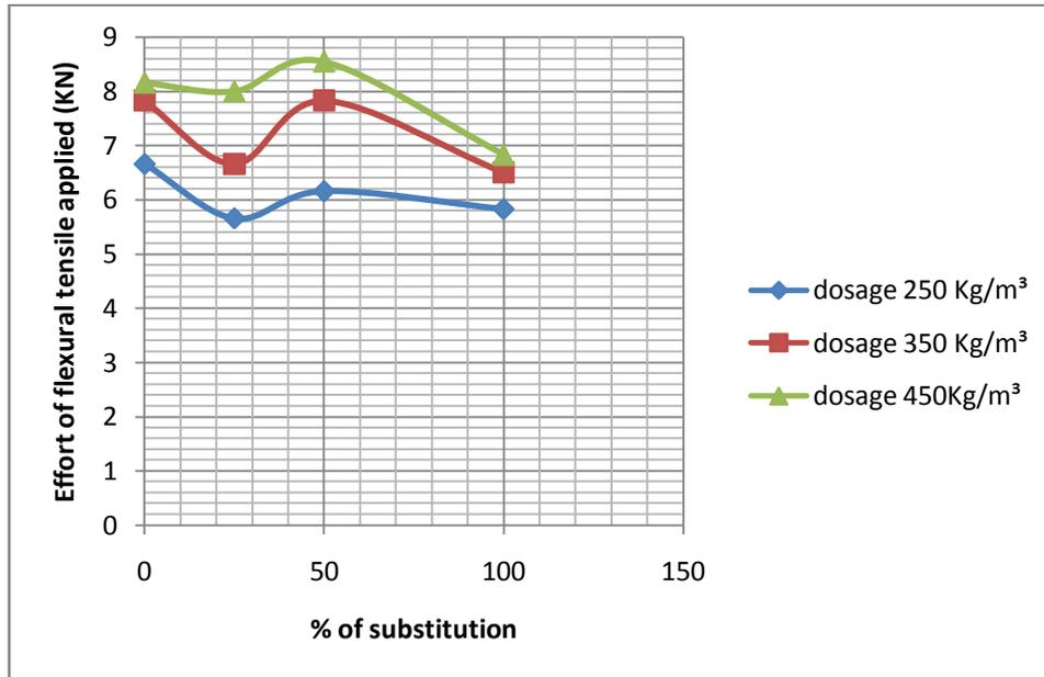
**Figure 5.** variation of the tensile strength of concrete at 28j according to substitution rate
