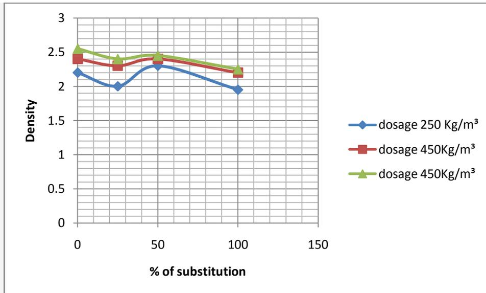
**Figure 1.** Variation of the density of fresh concrete in the rate of substitution
