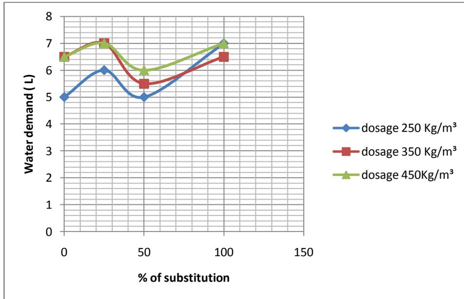
Figure 3. water demand of concrete depending on the rate of substitution
