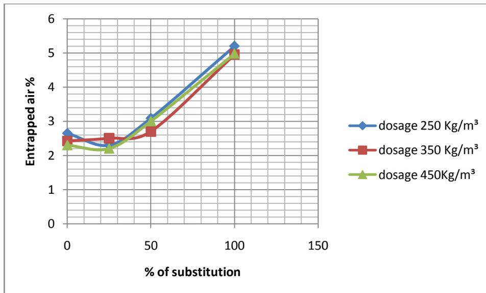
**Figure 2.** entrapped air concrete depending on the rate of substitution
