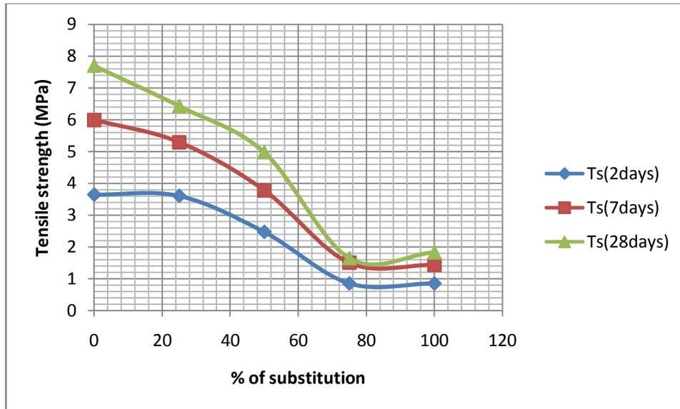
**Figure 7.** Change in tensile strength of the mortars according to the degree of substitution
