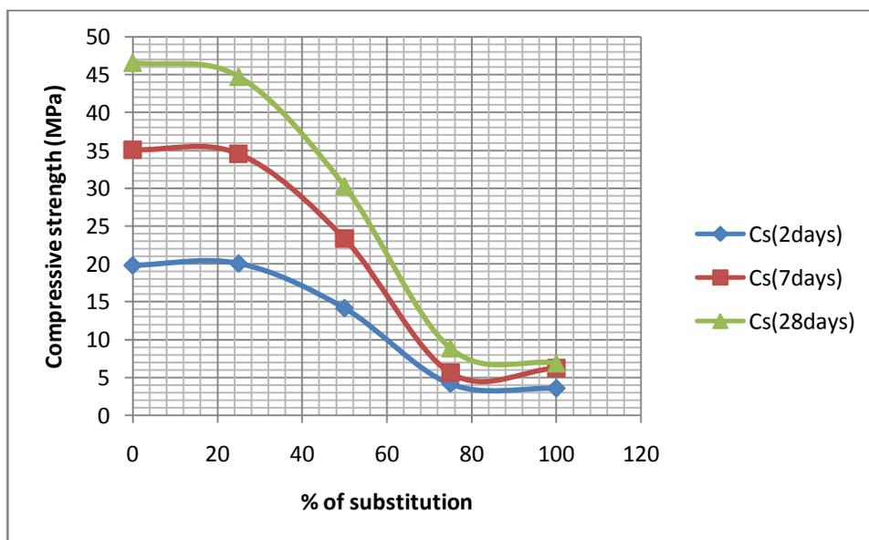
**Figure 6.** Variation in compressive strength of the mortars according to the degree of substitution
