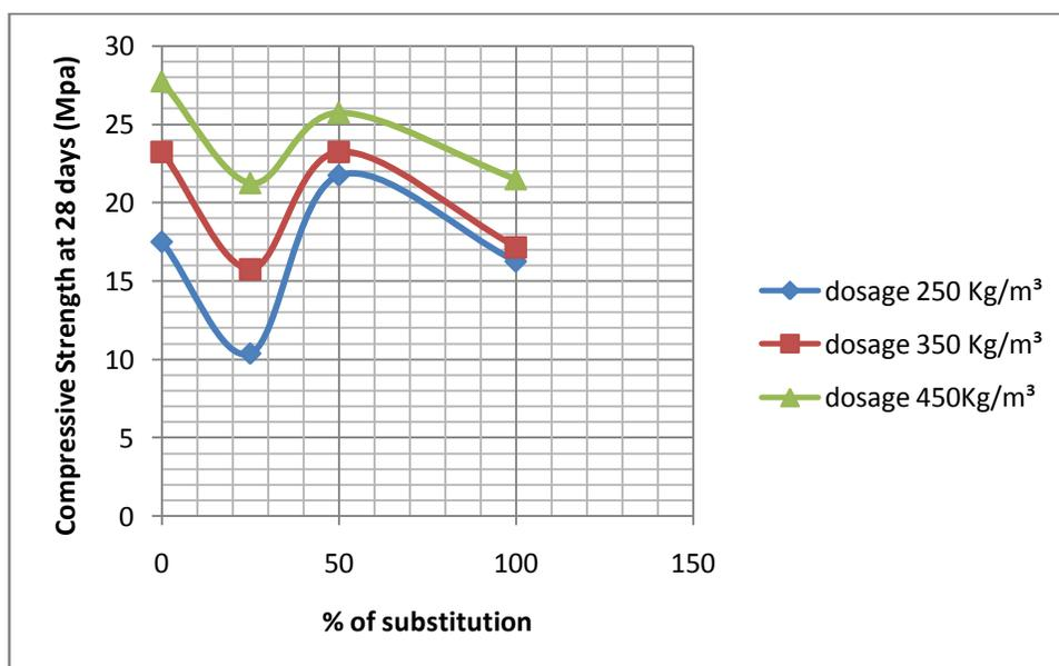
Figure 4. Varying the compressive strength of concrete at 28days according to rate of substitution
