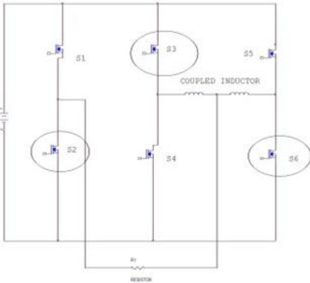
The figure shows diagram of proposed topology. The proposed system consists of the circuit implemented in closed loop. So an additional feedback signal is given to the circuit along with the pwm technique. So the waveform is obtained without shifting and correct output can be obtained. The obtained system is more stable as we get proper output.
