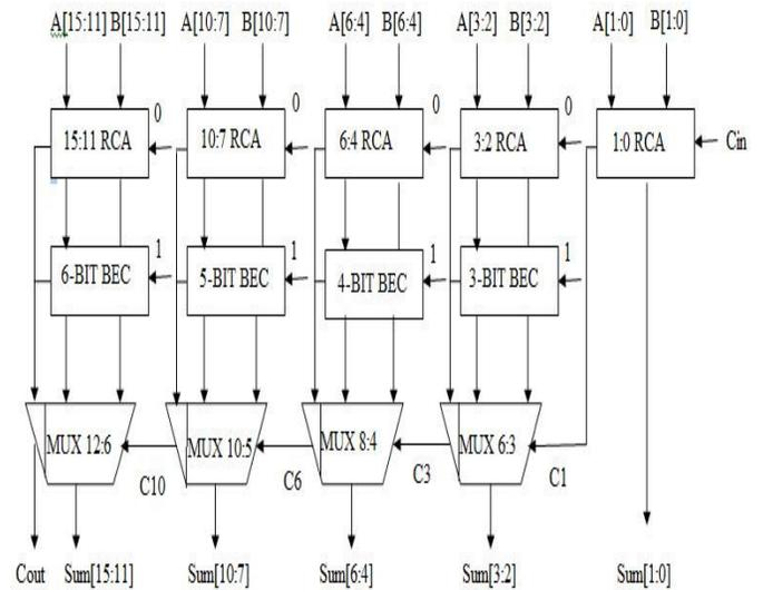
**Fig1: 16-bit Modified SQRT with BEC**
