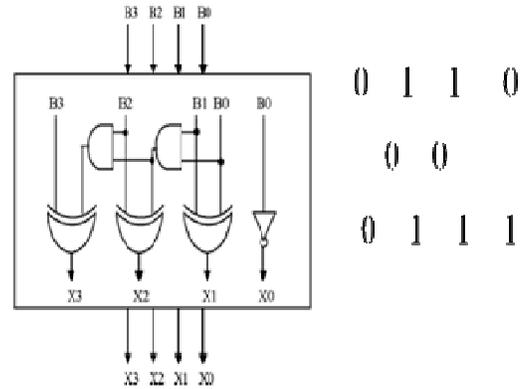
**Fig3:** Logic diagram of 4-bit BEC with example
