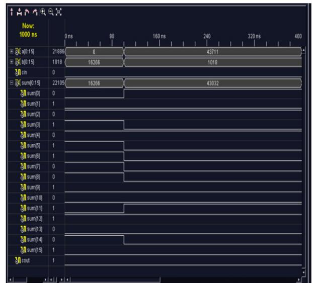
**Fig8: Output waveforms of 16-bit SQRT MCSA with BEC**
