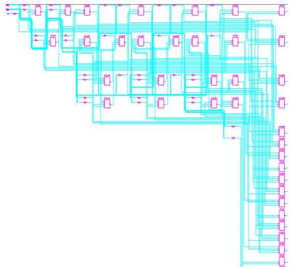
**Fig10:** Technology schematic of 16-bit Sqrt MCSA with CSA
