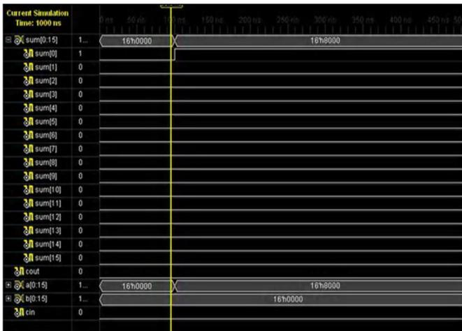
**Fig10:** waveform of 16-bit Sqrt MCSA with Carry save Adder.
