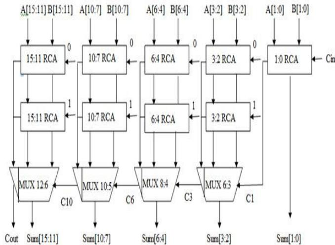
**Fig1: 16-bit SQRT with CSLA**
