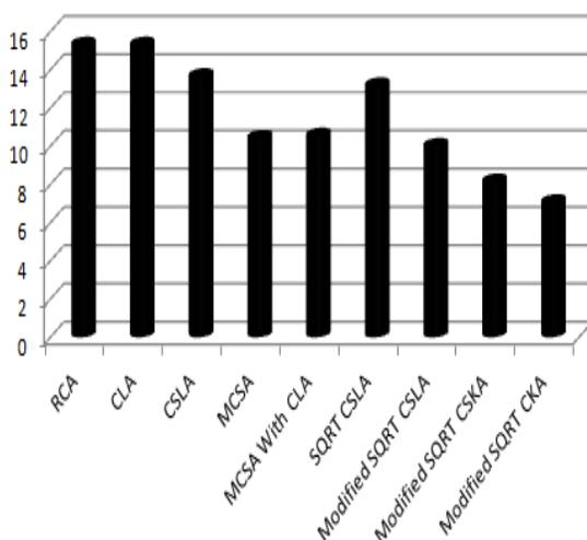
**Fig11.** Logical delay comparison of adders
