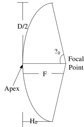
Fig.3. Geometry of the Prime Focus Parabolic Reflector Antenna
