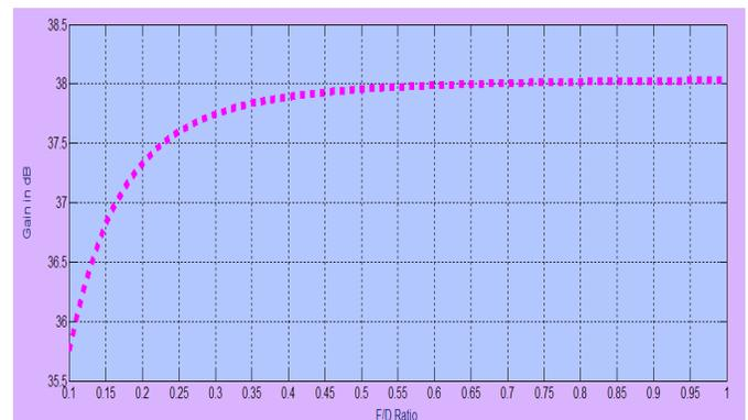
**Fig.9.** Plot of Gain as a function of F/D ratio
