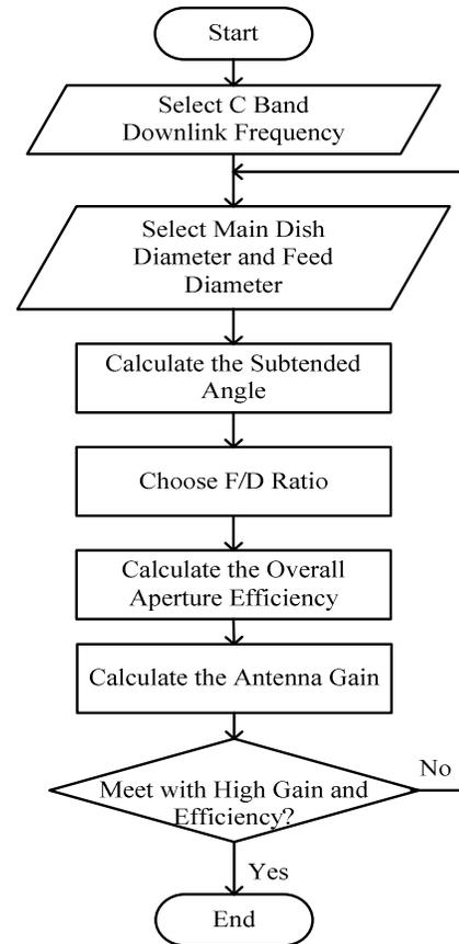
Fig.4. Flowchart of antenna gain and efficiency calculation
