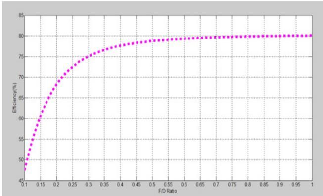
**Fig.10.** Plot of Efficiency as a function of F/D
