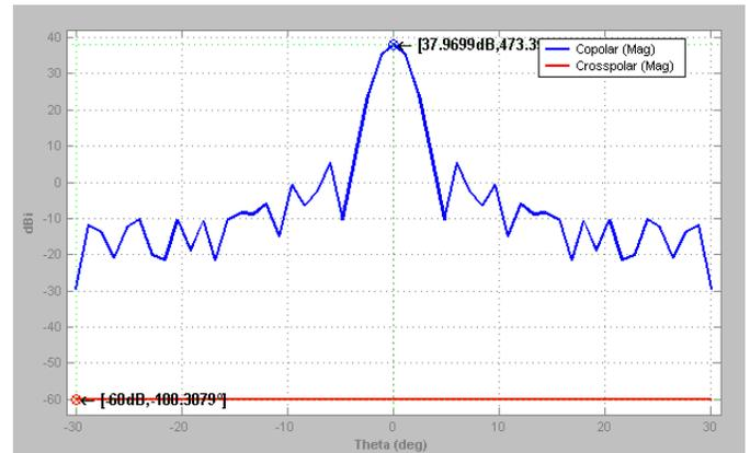
**Fig.8.** Far Field Phi Constant at 4.7215GHz
