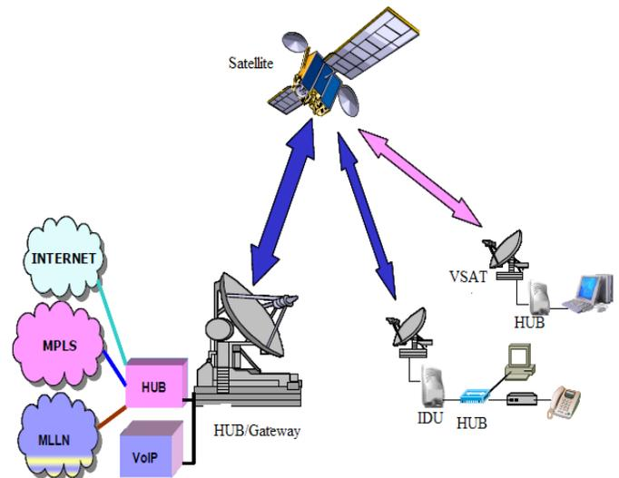
Fig.1. C band VSAT Architecture [12]
