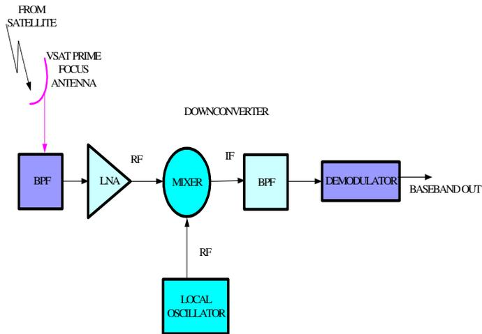
Fig.2. Block Diagram of VSAT downlink earth station system
