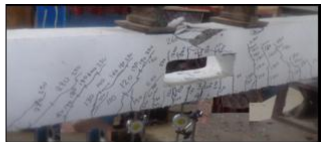
Figure (14) Crack Patterns and Load-Deflection Curve for Beam FBO1.
