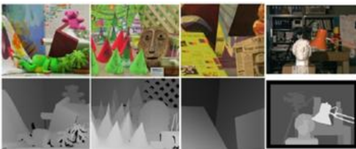
Fig. 1 Middlebury evaluation images (Top row), from left to right, Teddy, Cones, Venus, Tsukuba [1], Corresponding disparity map (bottom row).
