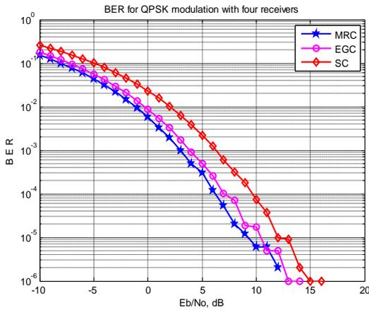
**Figure4.**BER performance with qpsk modulation in SC,MRC,EGC
