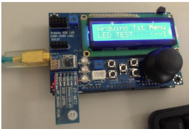
Fig. 3. The Arduino test platform for Bluetooth based LED control
