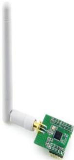
**Fig. 3** Zigbee Transmitter Module
