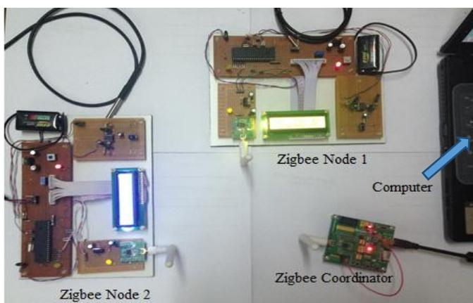
**Fig. 15** Experimental Test of Sensing Data from End Devices by Zigbee Coordinator
