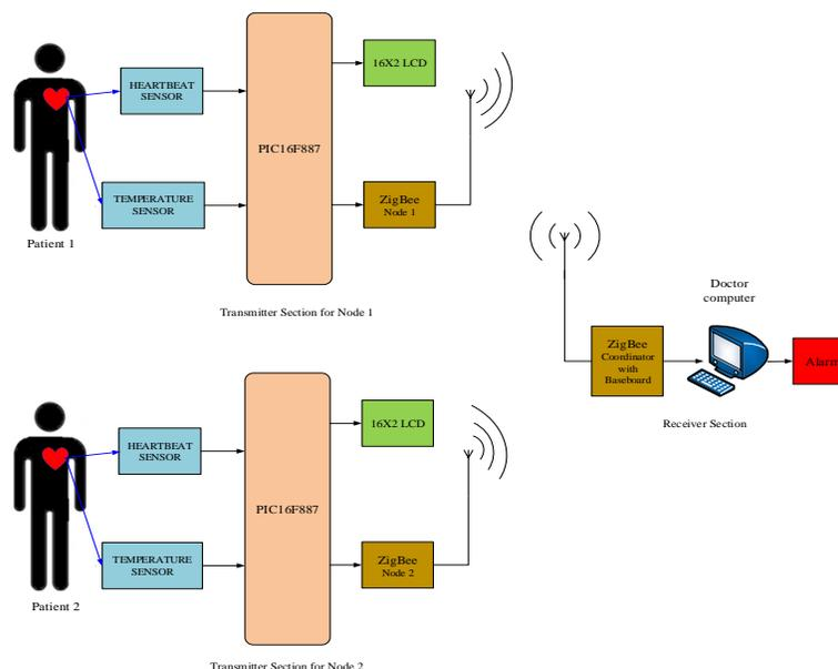
Fig. 1 Functional Block Diagram of the Overall System
