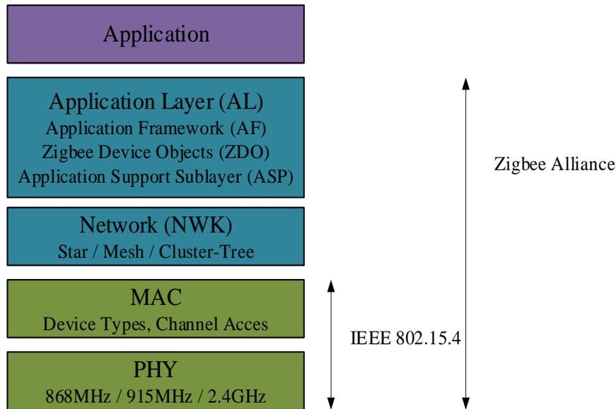
**Fig. 5** Architecture of Zigbee/IEEE 802.15.4
