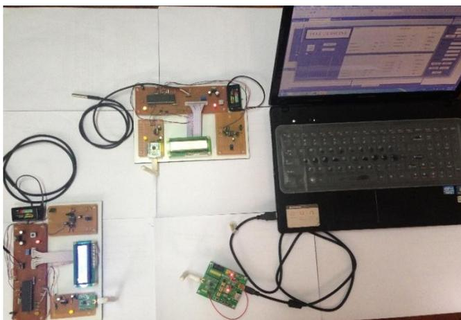
**Fig. 16** Experimental Test of Patient Monitoring System
