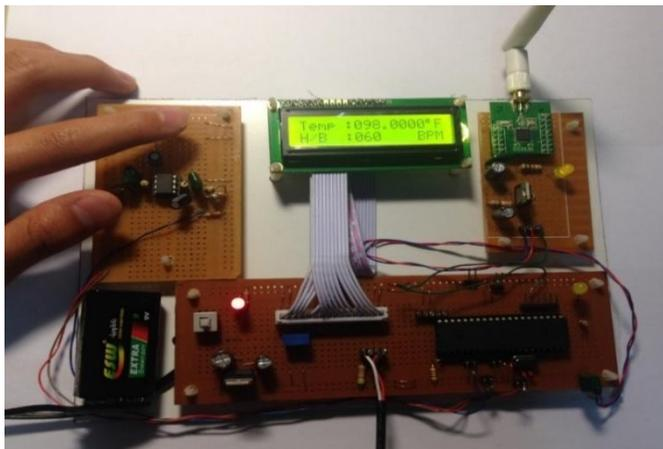
**Fig. 14** Experimental Test of Sensing Heartbeat and Body Temperature
