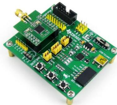
**Fig. 4** Zigbee Receiver Module with Baseboard
