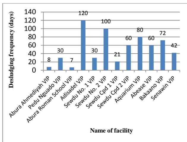
Fig 2. Desludging frequency (in days) of public latrines
