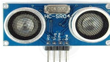
*Fig. 1 Ultrasonic sensor (HC-SR04)*
