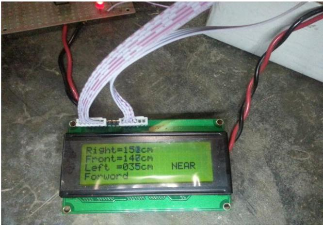
**Fig. 12.2** Test result for distance measurement of left obstacle with LCD display
