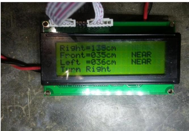
**Fig. 13.2** Test result for distance measurement of front and left obstacles with LCD display
