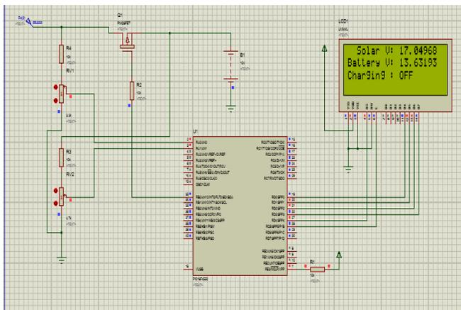
**Fig 8.** Simulation test for charging off when the battery is full
