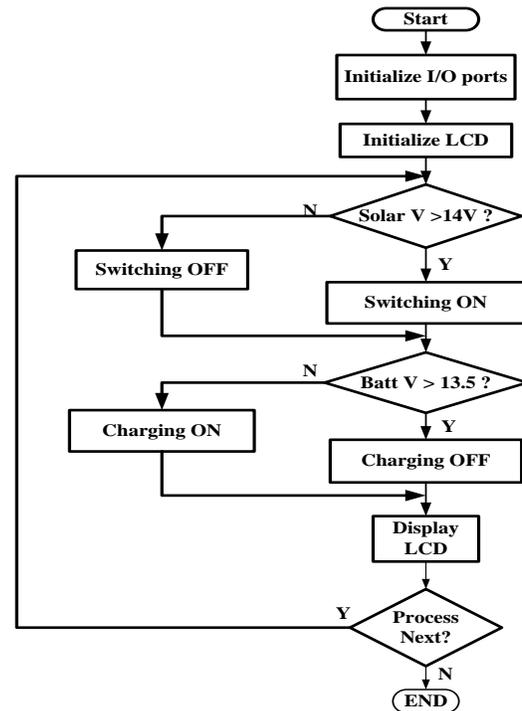
Fig 6. Flow-chart of battery charging system
