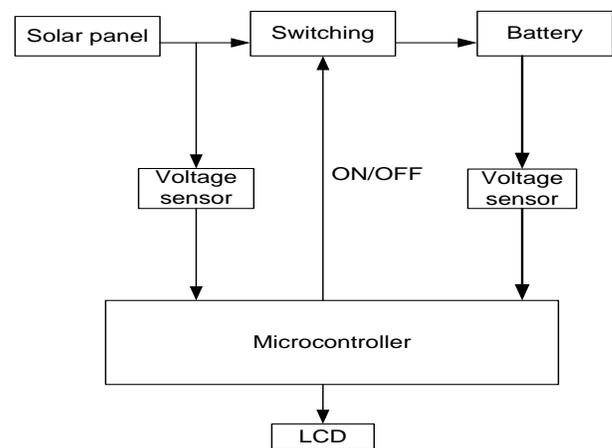
**Fig 1.** Block diagram of solar battery charger
