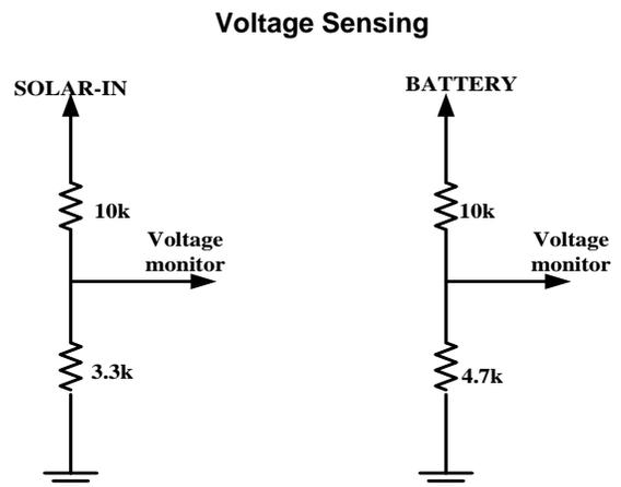
Fig 4. Circuit diagram of voltage divider
