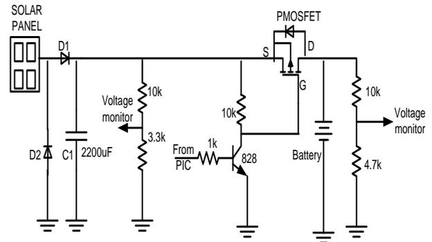
Fig 3. The circuit diagram of battery charger
