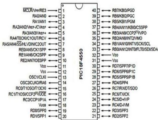
Fig 2. PIC18f4550 pin configuration
