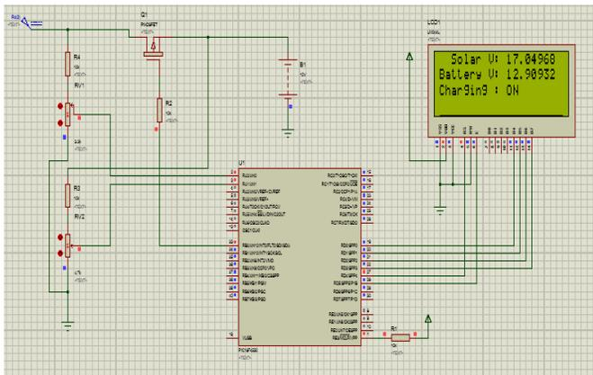
**Fig 7.** Simulation test for charging on when the battery is not full
